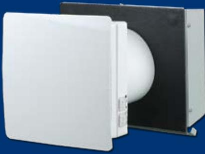
The ECO-FLO Energy Recovery Ventilator (ERV) is the all-in-one ventilation solution for new construction and renovation projects involving homes, apartments, or commercial buildings. The ERV core extracts thermal energy and moisture from the exhausted air, and uses it to pre-treat the incoming supply air.
