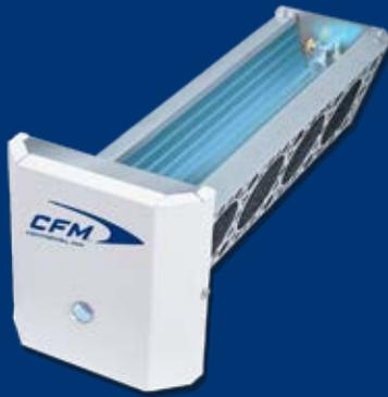
CX-Pro combines three powerful purification forces in an in-duct whole house air purifier. The UVC germicidal lamp neutralizes viruses, bacteria and mold. The patented design uses a Photocatalytic Oxidation (PCO) process to neutralize odors and toxic VOCs into benign constituents and an activated carbon adsorption media to trap odors and toxic chemicals.
