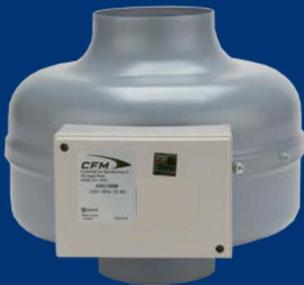
AXC In-Line Duct Fans are designed for residential, commercial and light industrial ventilation applications. The quiet, efficient backward-curved motorized impeller is capable of developing significant pressure, and the in-line configuration simplifies installation.
