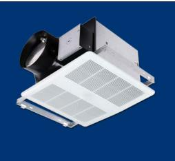
With its high efficiency DC motor, the TF140-DC Tranquil Bathroom Fan offers whisper-quiet exhaust that is under 1 sone, with multispeed capability. Toggle-switch positioning determines the maximum desired airflow rate, ranging from 90 to 140 cfm.
