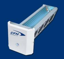
CX-Pro combines three powerful purification forces in an in-duct whole house air purifier. The UVC germicidal lamp neutralizes viruses, bacteria and mold. The patented design uses a Photocatalytic Oxidation (PCO) process to neutralize odors and toxic VOCs into benign constituents and an activated carbon adsorption media to trap odors and toxic chemicals.
