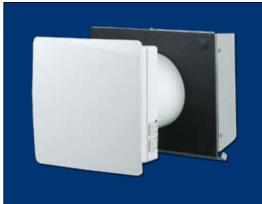
The ECO-FLO Energy Recovery Ventilator (ERV) is the all-in-one ventilation solution for new construction and renovation projects involving homes, apartments, or commercial buildings. The ERV core extracts thermal energy and moisture from the exhausted air, and uses it to pre-treat the incoming supply air.
