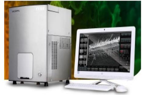
**EOI/EMCRAFT Scanning Electron Microscope:** The “Cube II” is an amazing new break through in the world of “Table Top SEMs”. With performance exceeding traditional analytical SEMs, it offers not only a smaller “foot print”, but unapparelled performance to larger SEMs.
