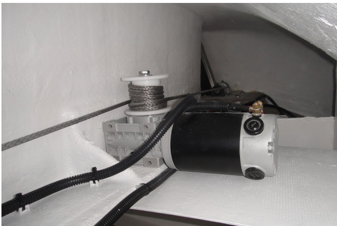
Pic. 18: Roof lifting system - winch.
