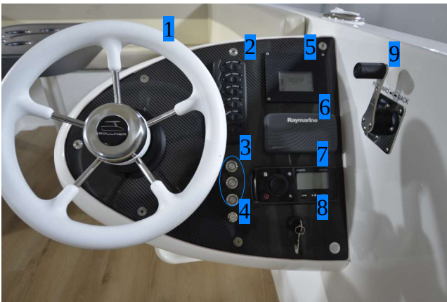
Pic. 24: Helm console - console device.
