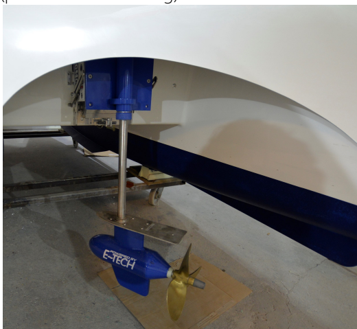
Pic. 12: E-Tech motor mounted on the transom.
