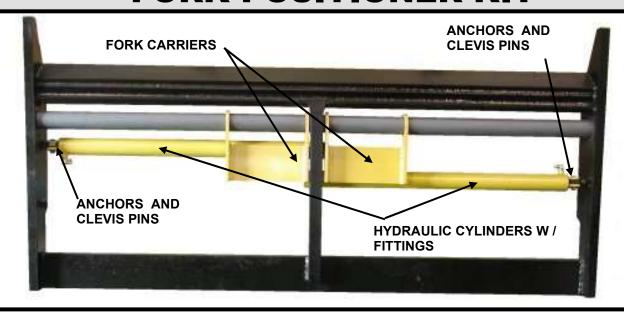
Convert Your Pin Type Carriage to Fork Positioning – reduce handling time. Operator stays on the truck and hydraulically positions the forks. Reduces operator fatigue and product damage. Requires one hydraulic function.
