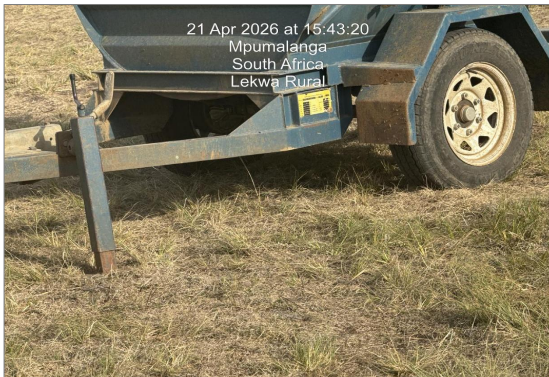
Figure 4: Machine standing without a drip tray.
