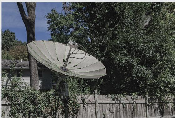
The SLS-FD6 is a lightweight 1.8m folding fabric parabolic dish with an integrated patch feed. The FD6 weighs just 10 lbs. and folds down to 8" x 8" x 52" for transport and storage. The integrated patch feed can remain in the dish when folded.
