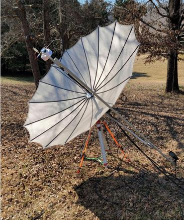
The SLS-FD8 is a lightweight 2.4m folding fabric parabolic dish with an integrated patch feed. The FD8 weighs just 15 lbs. and folds down to 8" x 8" x 66" for transport and storage. The integrated patch feed can remain in the dish when folded.
