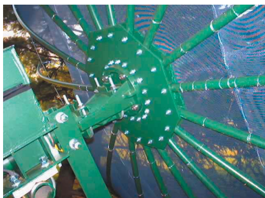
Figure 7 a). Back of dish – note wire for attaching mesh b) Mounting wheel details
