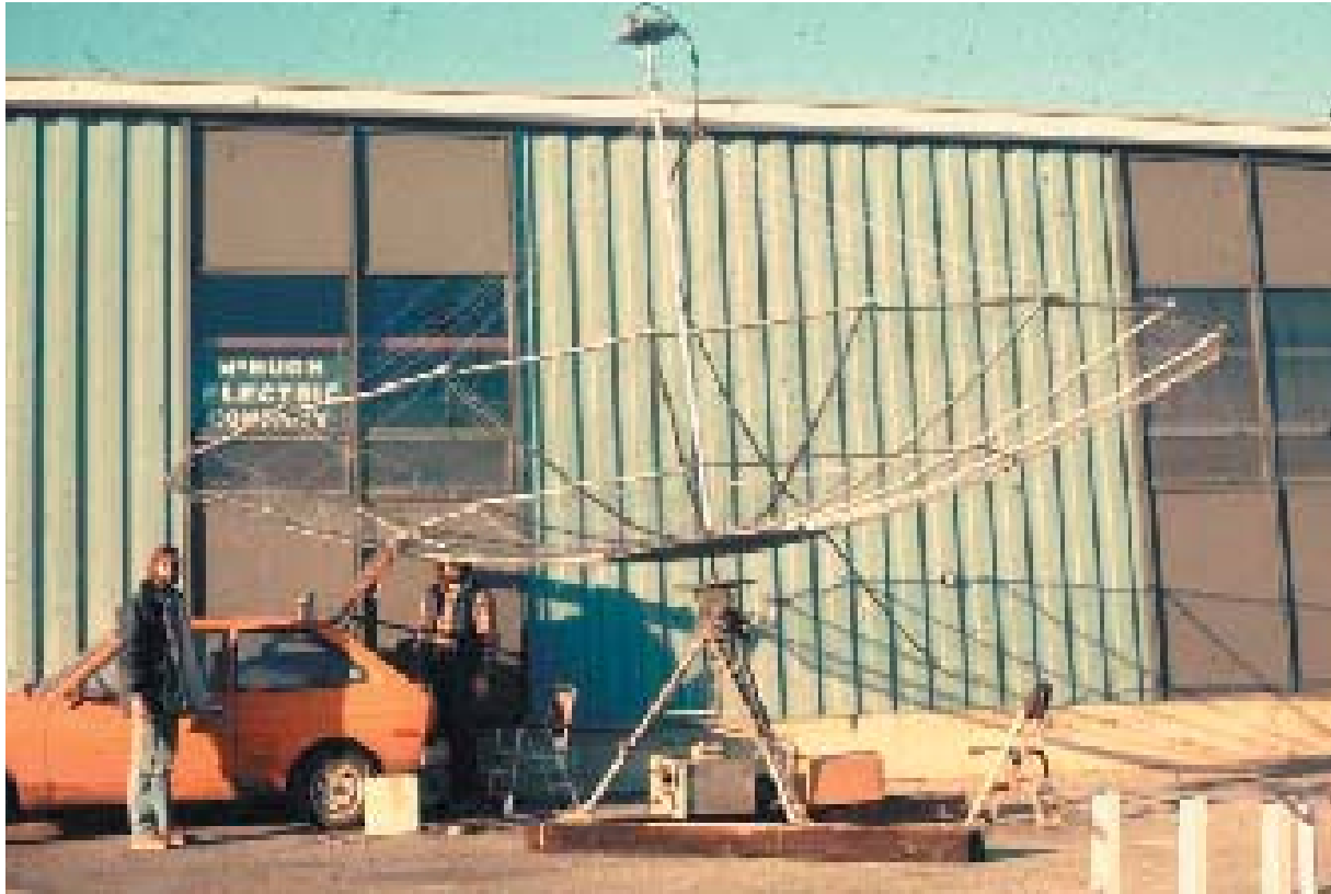
Figure 8 Portable 20 foot stress dish in DE. Carried on top of car
