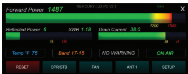
Figure 5 — The companion Windows PC software replicates most of the indicators and control buttons on the front panel.
