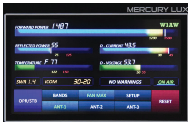
Figure 1 — A 7-inch high-resolution color touchscreen dominates the front panel. All monitoring and control, except for the power switch, are handled on-screen.
