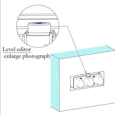
5. Adjust the embedded body (have connected all pipes) on the horizon line, and then screw the expansion bolts into fixed male screws to fix the embedded body. After that, open the water to test if all pipes have leakage or not and all water functions work well. At last, seal the wall.
