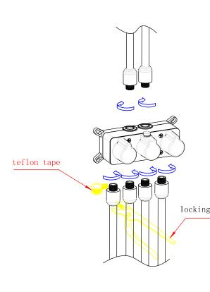
4. Please flush all pipelines to ensure that there is no debris such as downstream sand and gravel before connecting the shower. And then wrap hot & cold supply water pipes (not provided)
