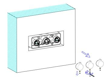
7. Remove three plug from handwheels first. Use 2.5 mm hexagon to loosen the three handwheels at counterclockwise direction, and take them out. Don't get off Wearing ring
