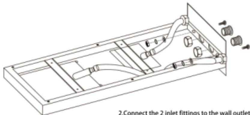
2.Connect the 2 inlet fittings to the wall outlet fittings; then install the nuts, expansion screws and inlet pipe.
