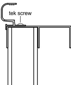
**Radiant Concrete Receptor Coping**
