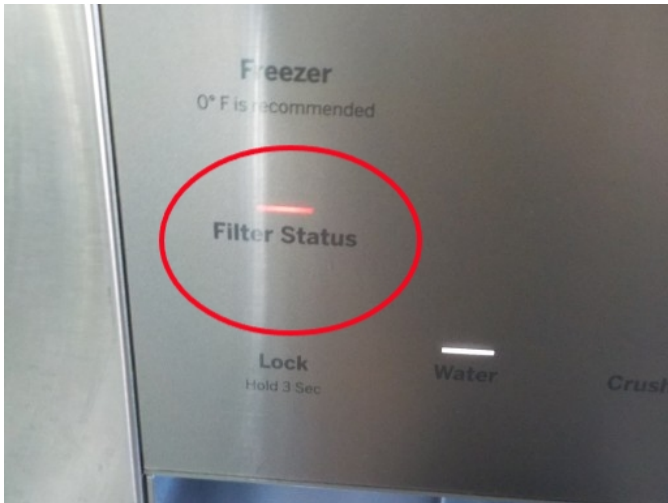
Filter will need replacement
