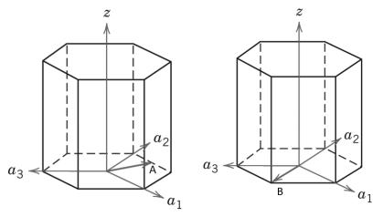
(b) Determine the indices for the planes A and B shown in the following hexagonal unit cells
