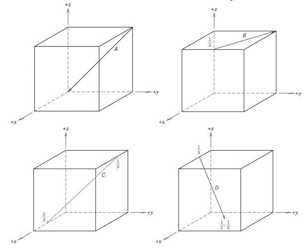
8. Determine the Miller indices for the directions shown in the following cubic unit cell
