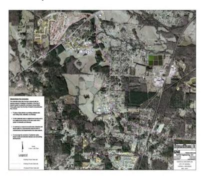
GNE was selected by the City of Haskell to assist in the preparation of a sidewalk master plan. The purpose of the project was to create an inventory of existing sidewalks and prepare a plan for the expansion of Haskell's sidewalk system to promote non-vehicular transportation. Haskell intends to use the master plan as a tool for attracting grants and other funding for these types of projects.
