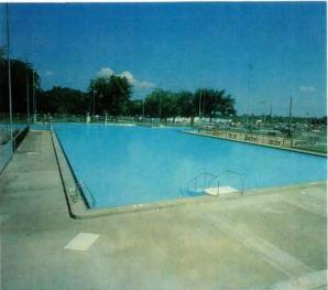
Suspended pool built over a hi-rise garage. Steps were prefabricated from fiberglass, set in place and laminated. The entire pool, including the overlow gutters and deck edge were laminated; overflow gutters and step risers were painted in a contrasting color.
