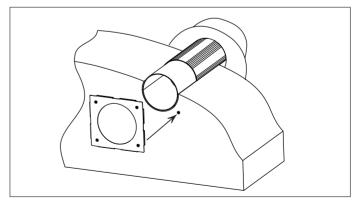
Caution: The ventilator must not be installed in a location where the air duct will be obstructed by curtains, blinds or other item that can interfere with the air flow.
