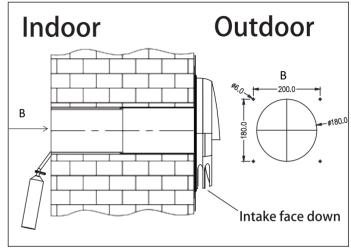
4. Paste the location sticker onto the wall surface, paying attention to the direction ensuring the circle marked on the sticker lines up with the duct. Mark the drilling hole positions and remove sticker. Drill 4 x 6 mm holes and fill holes with rubber wall plugs (supplied).
