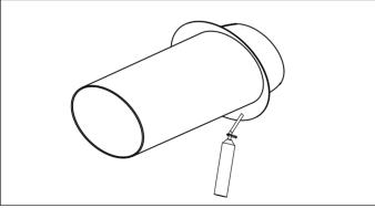
3. Pull back the duct through the wall hole to make the inner side rubber ring fix to the outside wall. Fill the gap between the wall and duct with foam glue. The inner duct should be perpendicular with indoor wall surface.
