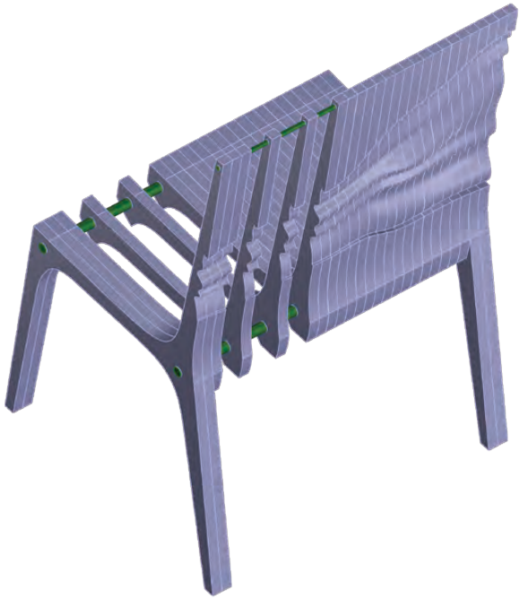
Materials Used: 24 CNC Milled Profiles, 3/4” Birch Plywood Sheet, 3 Wooden Dowels, Clear Coat Polyethylene Exploded Axonometric Assembly - Iggy So (Below) Conversation between Achilles and the Tortoise- Iggy So+Faris Faraj (Right, Foreground) Worm’s-Eye Isometric Rendering of Normals - Iggy So (Right, Background)
