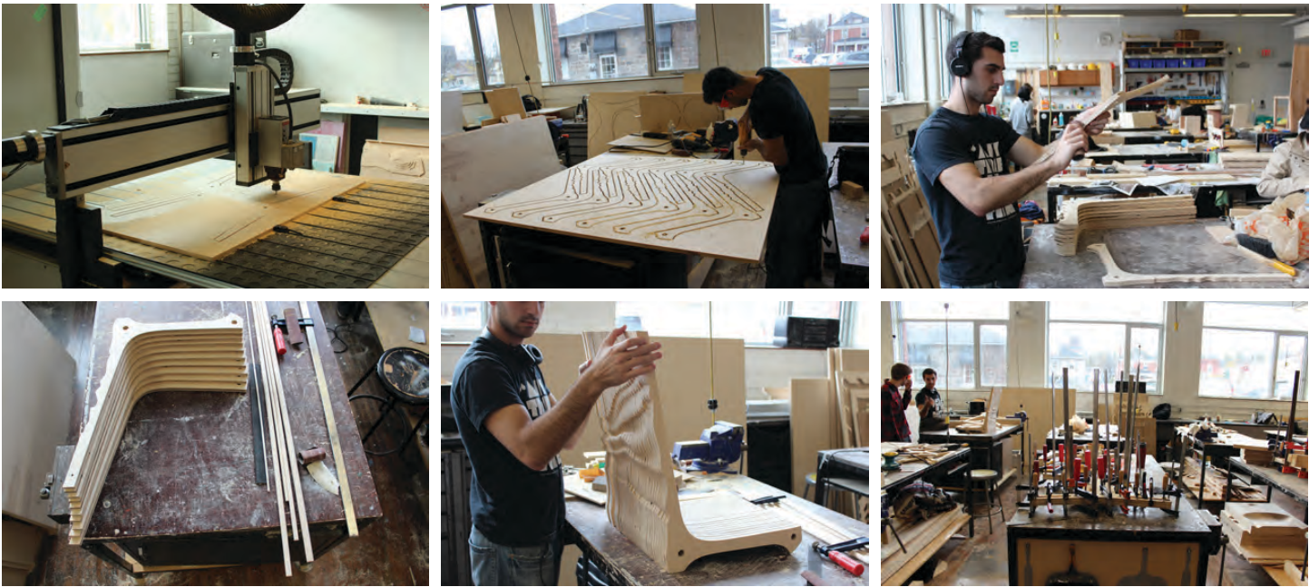
Process Documentation (Above) CNC Milled Profiles - 4 Hours Manual Trim Routing Sanding Threading Clamping & Lamination
