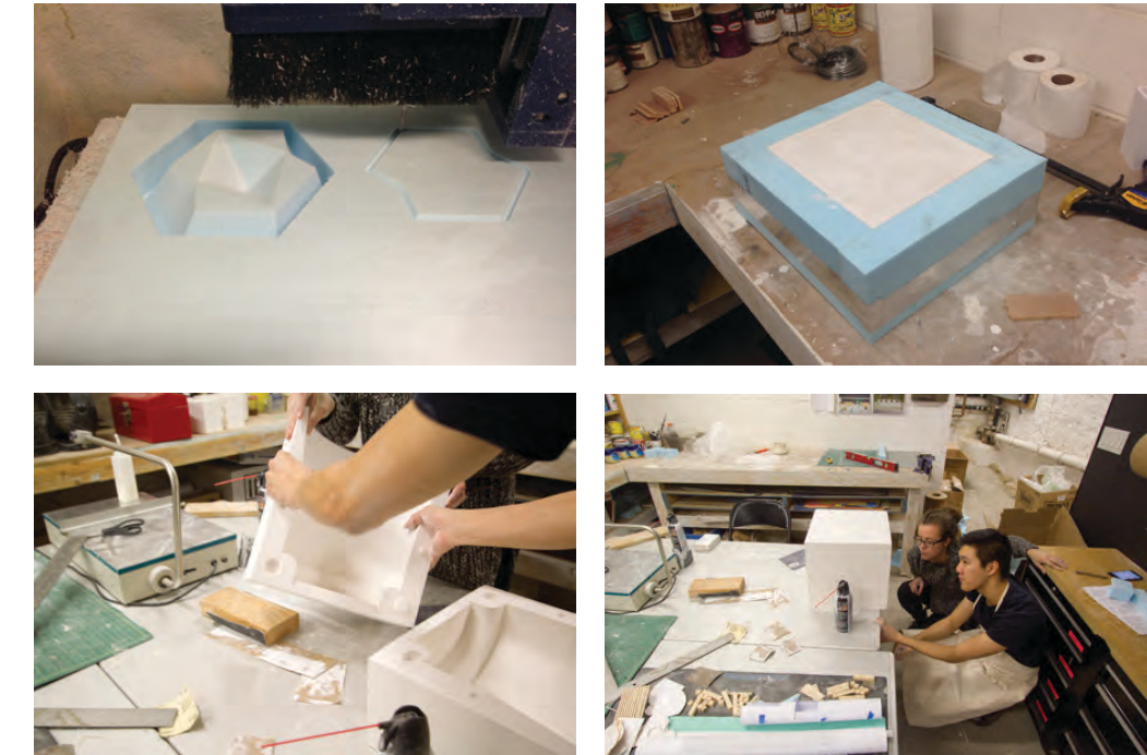
Ceramic Fabrication Process Work. CNC Milling; Plaster Pour; Sanding; Fitting - Iggy So + MOS (Left) Completed Ceramic Vase and Tray - Iggy So + MOS (Bottom) Rendering from Obama Presidential Library Competition - Iggy So + MOS (Next Page, Top) Axonometric Drawing from Ordos House Proposal - Iggy So + MOS (Next Page, Bottom)
