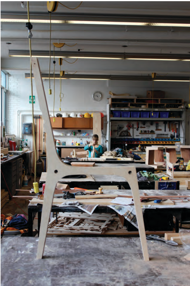
Materials Used: 24 CNC Milled Profiles, 3/4” Birch Plywood Sheet, 3 Wooden Dowels, Clear Coat Polyethylene Exploded Axonometric Assembly - Iggy So (Below) Conversation between Achilles and the Tortoise- Iggy So+Faris Faraj (Right, Foreground) Worm’s-Eye Isometric Rendering of Normals - Iggy So (Right, Background)
