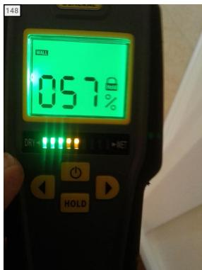
Evidence of prior water leak- tested dry
