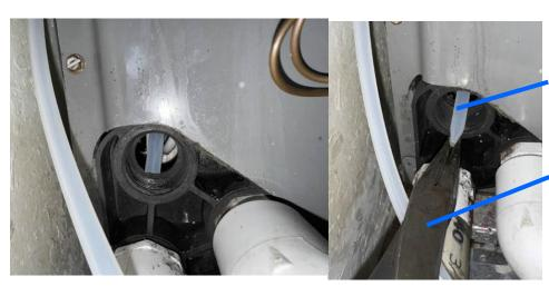
The plug was removed and the 380mm (15") dispense tube was lowered behind the stationary panel to the drain outlet, and the tube was pulled out with a needlenose pliers
