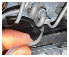
The two right coils share a common drain trough so either location can be used. I decided to go under the coil instead of routing the tubing up over the front plate and then back down to the back of the "V."
