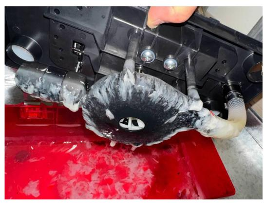
I vacuumed out the pump and cleaned the Zoog with paper towels. The tank has a solid film stuck on the bottom and sides.
