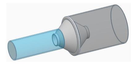
The Vacuum Adapter Holder's tapered opening matches the Vacuum Adapter's cone tapers, thereby providing a high contact surface area for a superior seal, and for nesting the vacuum adapter in the holder during storage:
