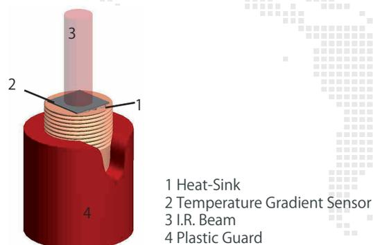
In fact, the temperature reached by the top surface of the sensor attains few degrees Celsius over the heat-sink temperature and hence involves negligible convection and radiation losses.
