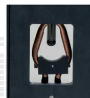
The **mechanical stimulator** relies on thin wires attached to a mounting plate. The system comes with several plates, each with a different number of wires in order to apply different force levels to the animal vibrissal pad.
