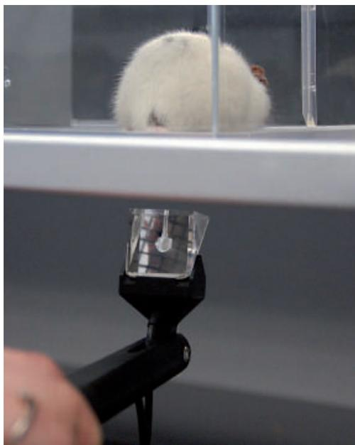
Fig. 1: "touch stimulator" with prism. Optional grid mesh not included
