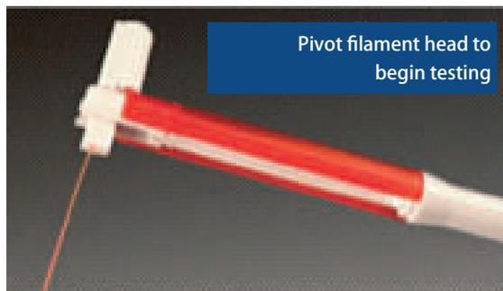
Pivot filament head to begin testing
