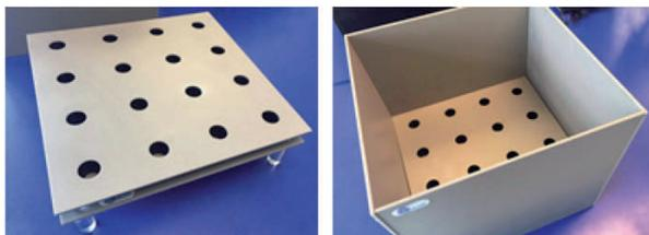
The **46653** is a simple open field, dimensioned 40x40cm, with 16 holes diam 3cm, spaced 10cm apart (from center to center), enclosed in transparent (or opaque) walls. The non-reflecting surface makes it particularly suitable for Videotracking.
