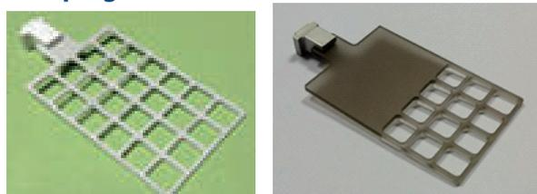
Grasping-grids are also included, for integrated measurement of the four limbs (left) or hindlimbs (right).
