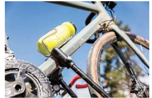
UPRIGHT ARM CONNECTS TO DOWN TUBE
