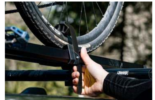
RATCHET STRAP SECURES REAR WHEEL
