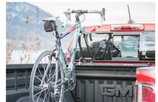
THE TELESCOPING BAR EXPANDS TO FIT MANY TRUCK BOX WIDTHS
