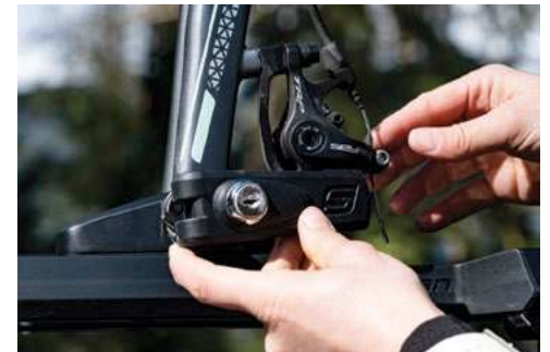
INTEGRATED LOCKING 9 MM FORK MOUNT
