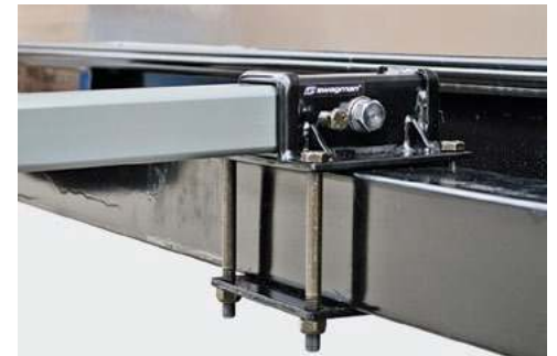
ADAPTER PROVIDES A SECURE WAY TO CARRY AN RV APPROVED HITCH BIKE RACK
