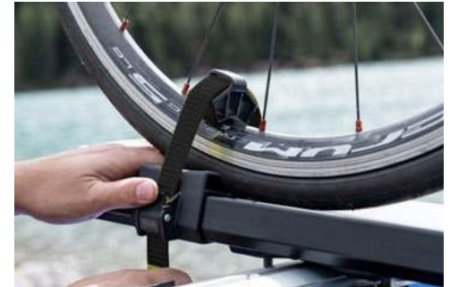
RATCHET STRAPS FIRMLY HOLD WHEELS
