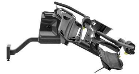
TILTS DOWN, WITH BIKES ON TO ALLOW ACCESS TO REAR OF VEHICLE
