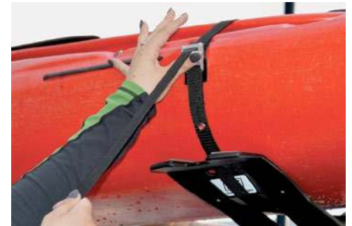
TIE DOWN STRAPS SECURE BOAT TO RACK
