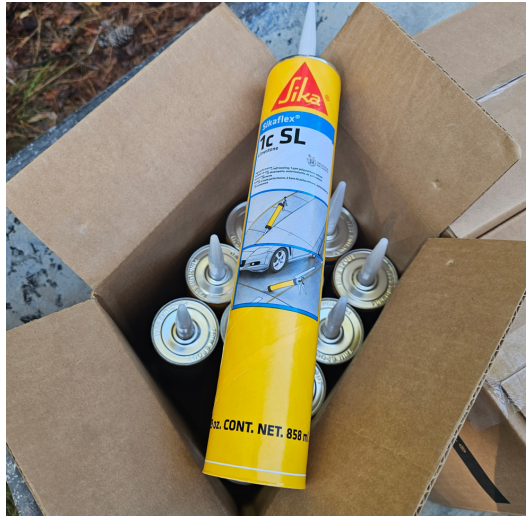
Figure 10 – Caulk used to seal the gaps in the slopes of the spillway
