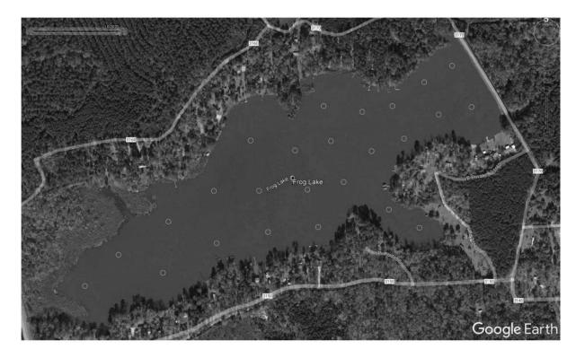
The system would consist of a single compressor with 13 hp motor. It would be installed in an 8' x 8' shed or similar enclosure (excluded from Clean-Flo's scope). There would be 25 12-inch diffuses distributed throughout the lake, connected to the compressor with 5/8" self-sinking airline. We recommend that a season program of bio augmentation be followed in addition to installing and operating the diffusion system. A preliminary system layout is attached. Budgetary Costs are as follow:
