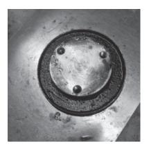
Example of a swivel that was not lubricated regularly and that accumulated sand within it.
