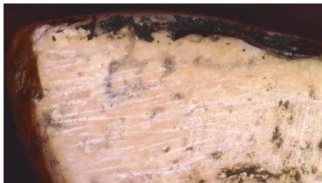
an edge: file and sanding scratches
