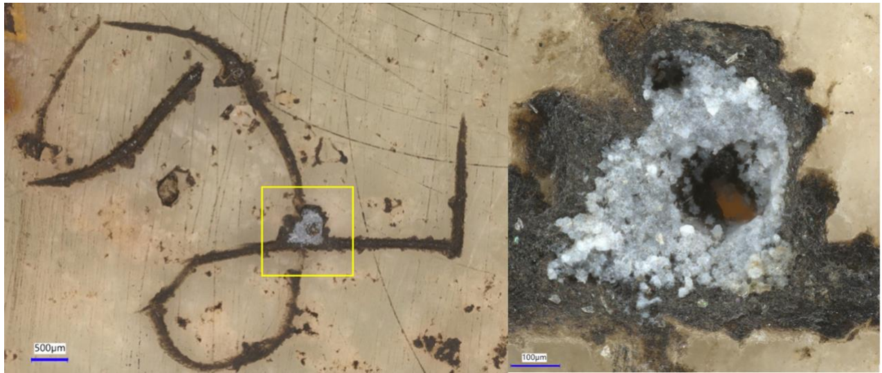
Figure 47: Artifact E micrograph, ultra-fine detail surface engravings with embedded efflorescence crystals.
