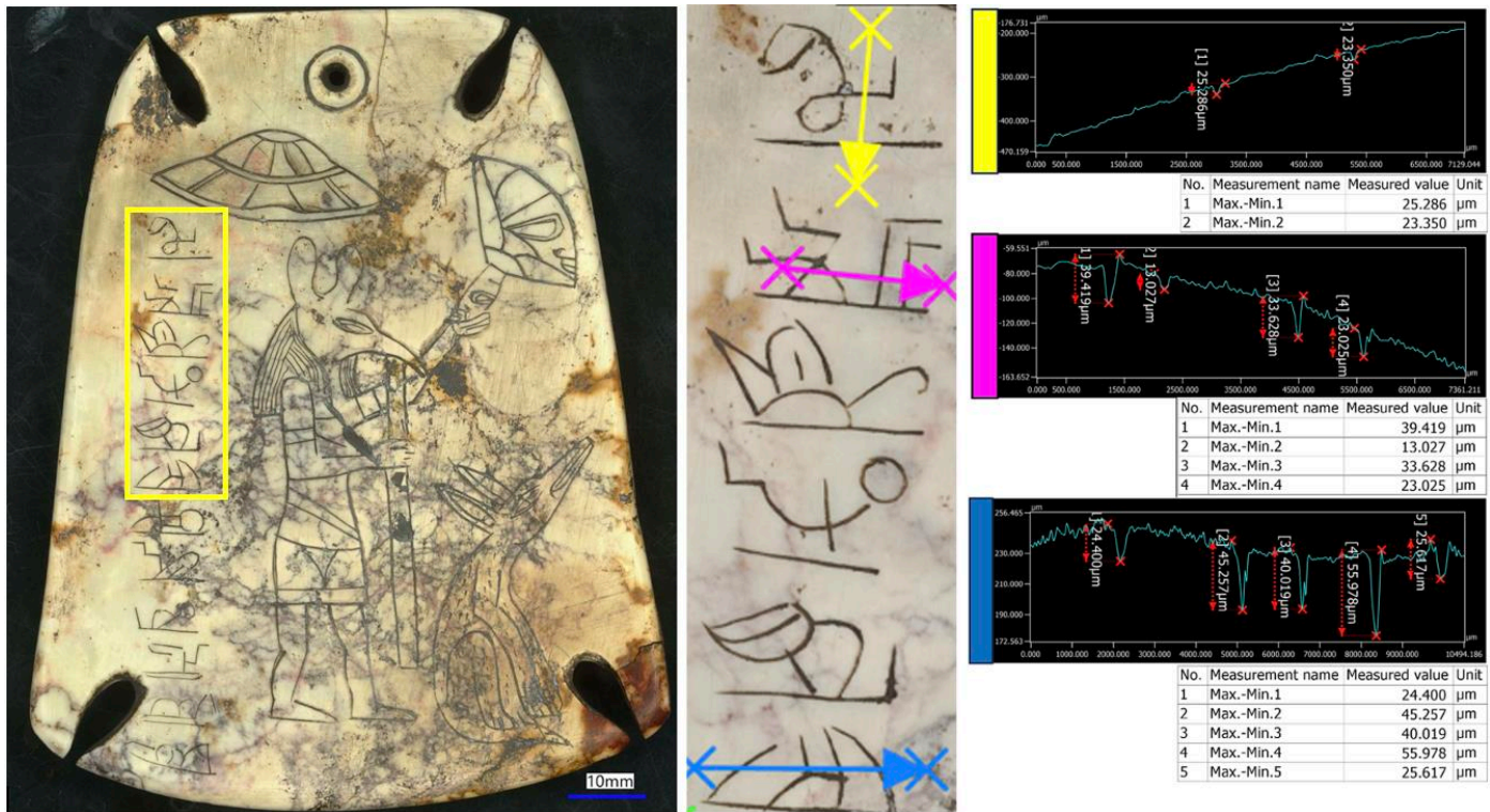
Figure 49: Artifact E, front side, \sim 30 \mu\text{m} engravings measured by high resolution surface texture mapping.
