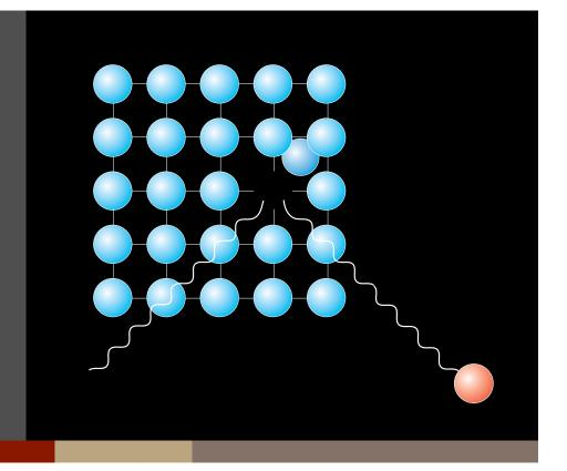
are often unstable, emitting alpha particles as they decay. These alpha particles, or helium atoms, get trapped in the material, which can affect its weldability for performing repairs, thus necessitating the replacement of failed components.
