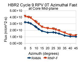
FIGURE 1. Comparison of RAMA and RNP-F Fast Fluxes at RPV Inner Surface at Core Mid-plane
