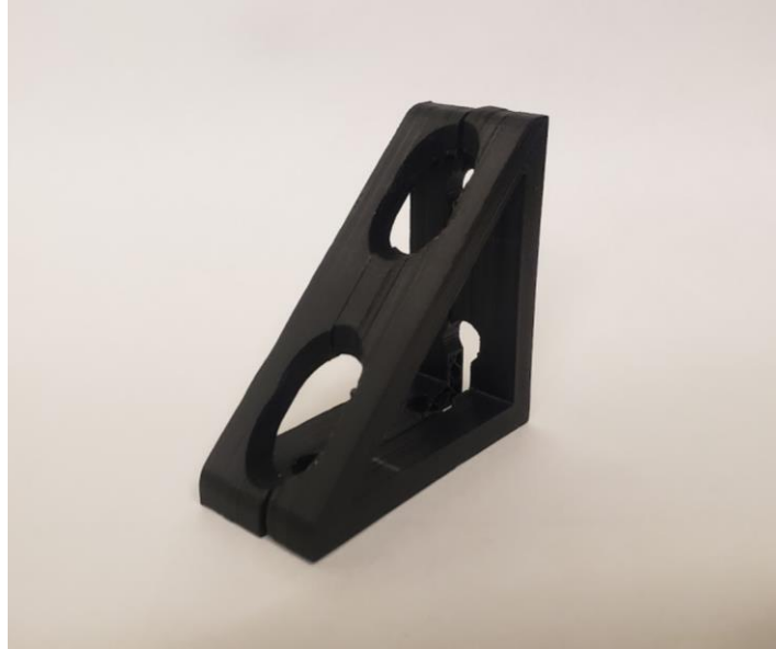
Figure 29: Photo of a 3D printed bracket with a 20% infill with printed holes. Note that this bracket split down the middle where the holes were.
