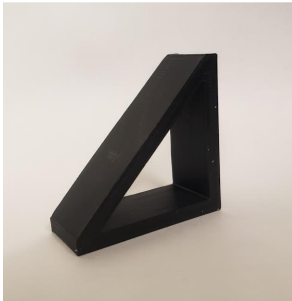
Figure 30: Photo of a 3D printed bracket with a 100% Infill with no printed holes. Note that the holes will be drilled through the bracket.
