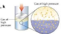
When the gas is compressed, gas molecules enter the liquid more frequently, so more are dissolved
