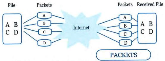
(U) When files are transmitted across the internet, they are broken into chunks, called packets, which are individually routed to the final destination and reassembled when they get there.
