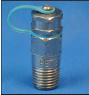
Product: #400 Core: Neoprene Thread: 1/4" NPT Length: 1 1/2"
