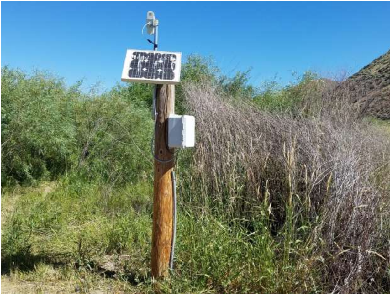
The photos on this page show the telemetry station which was installed in Pegram. This telemetry station is solar powered and provides up to the minute flow data to the landowner, helping to also ensure that the proper amount of water is being used in the irrigation canal. The lower photo shows the probe that sits in the bottom of the stream and sends information back to the computer mounted on the pole, SC Photos.
