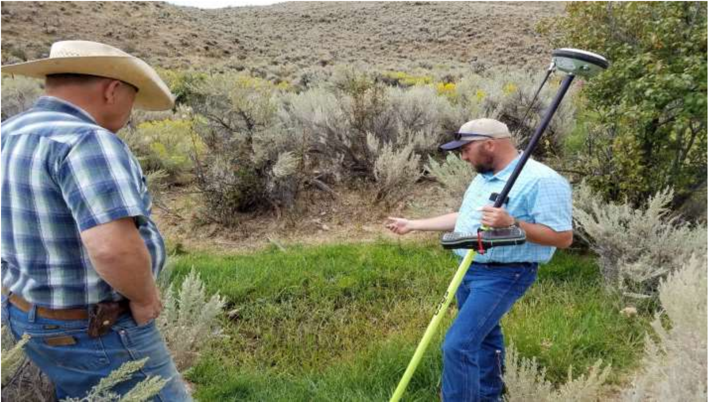
This photos shows ISWCC Engineer Allan Johnson discussing the route of a stockwater system, as we surveyed the elevations and topography to ensure the system would work properly after installation, SC Photos.
