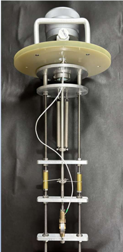
The MR Calibrator designed for use with LN2 or LHe open-mouth dewar
