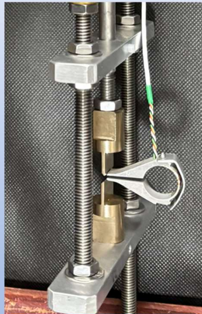
Knife edge hardware for calibrating COD Gages and Flat Tensile Extensometers
