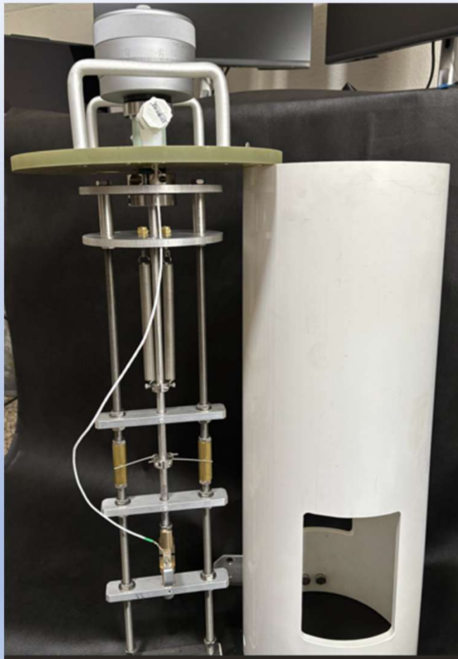
Calibrator shown next to the room temperature calibration/storage tube
