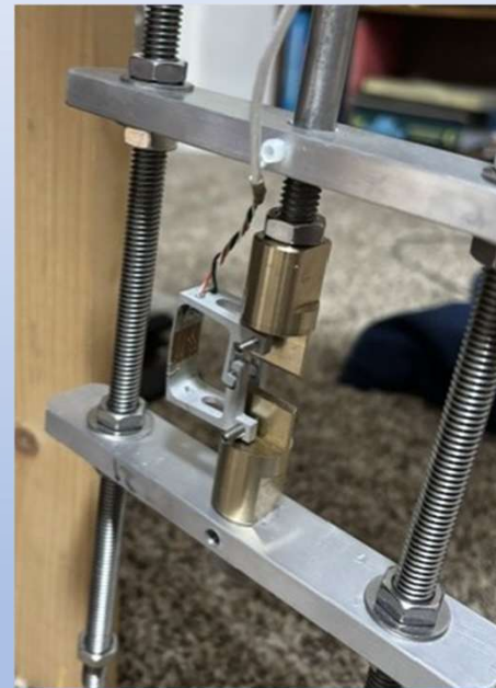
Knife edge hardware for calibrating COD Gages and Flat Tensile Extensometers
