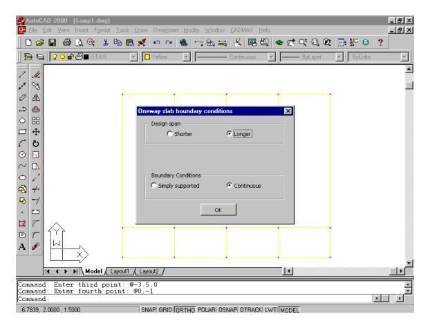
Select the longer span as design span for staircase flight slab and then press OK to complete command. Now you will see a flight slab is drawn in the drawing in the layer STAIR.
