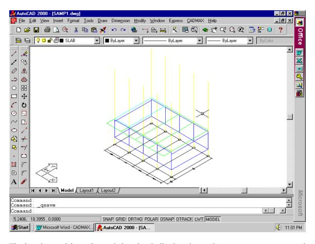
The last drawn slab can be copied to the similar locations using copy or array command as shown below:
