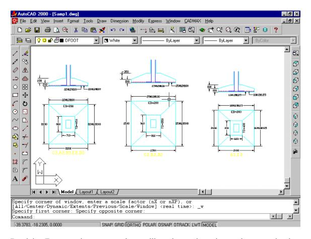
By giving Zoom previous command you will get the previous view as shown previously. Now you can make "OFF" the layers "DFOOT" and "FOOT" and set the current layer as "COLUMN" or "BEAM" or "GBEAM" since the detailing of footings is completed. Now you will see the screen as shown below:
