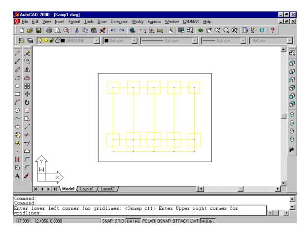
After the selection set is released, the Gridlines according to our option will be drawn in the drawing as shown below. The grid line notations written within the circles will be drawn in a separate layer "GRIDLINE" automatically so that you can "ON" or "OFF" the "GRIDLINE" layer as per your requirement.
