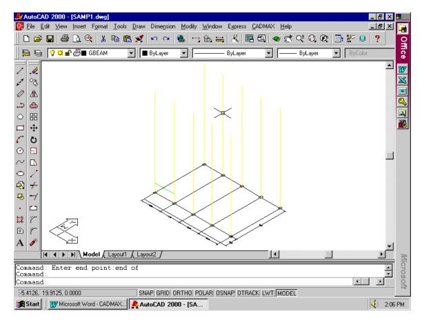
After drawing the first grade beam to adopt similar beams at other places you can copy or array the last drawn beam as given below:
