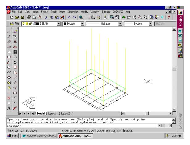
Now to introduce walls supported on the grade beam use the wall command as follows: **4.**Pick the "WALL" command in the CADMAX Pop-up menu.
