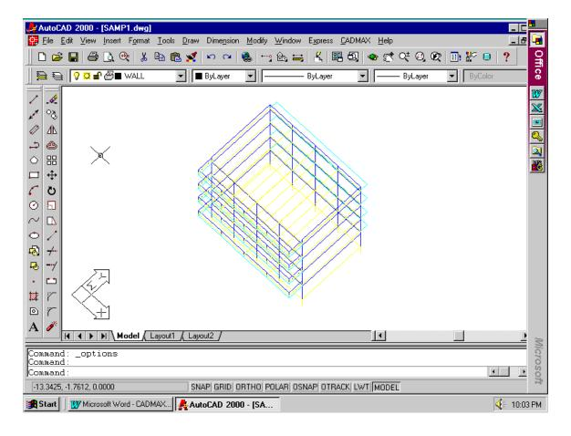
Now the structure is ready for analysis. Before analysis of the structure as a whole, the edge beams in the front side of the structure is to be analysed to get the point loads trasmitted to the cantilever beams. Since the loads from walls and slabs were transferred to the beams the layers containing walls, slabs, facia etc. may be off. Using the following dialog procedure.
