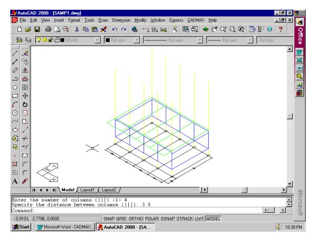
Now all the beams at floor level are drawn and now the slabs between beams are introduced as follows:
