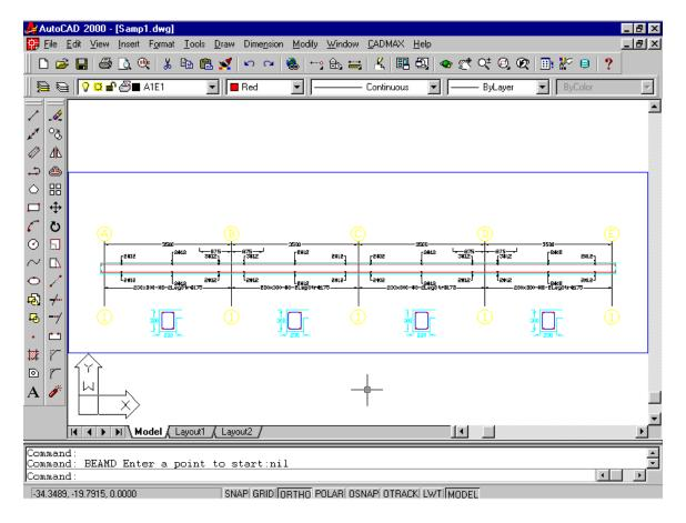
Similarly for other beams also detailed using "BEAMDSEL" and "BEAMD" command as detailed below:
