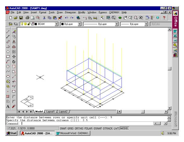
Similarly you can draw the beam at floor level in Y-direction using the **BEAM** command from **CADMAX** Pop-up menu. Enter the layer name to draw as **BEAM** and fill in the dialog box for beam details as given below and then **click OK**.
