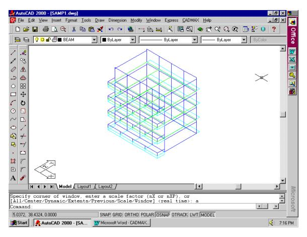
Now you can turn ON the layers "COLUMN,GBEAM,GWALL" for proceeding further. Now the drawing will be as shown below. Please note that the layer "0" is turned "OFF" for further analysis purpose.
