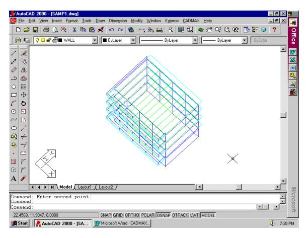
Now you copy the last drawn wall to the right end using copy command. And you can draw similar parapet walls in rear side also using the same wall command and then copy or array command. Now you will see the final structure as shown below.
