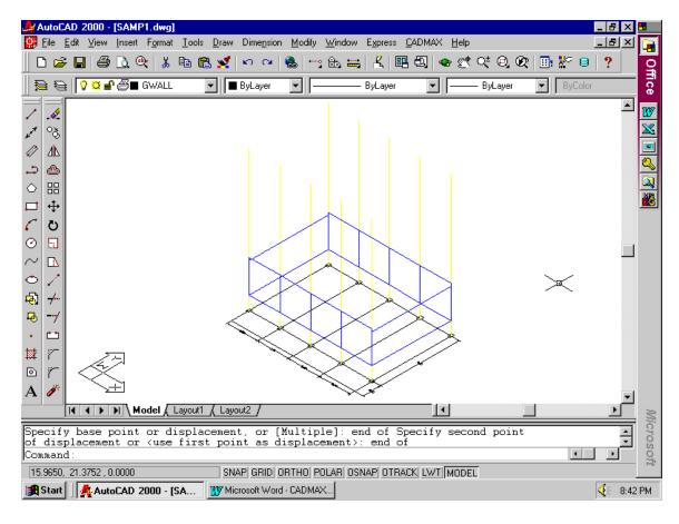
Now the grade beams and walls supported on the grade beams are introduced in the structure. Now let us insert the floor beams, slabs and walls as follows.
