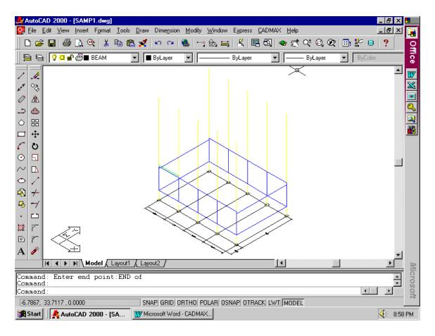
Give array command as follows to copy the similar beams.
