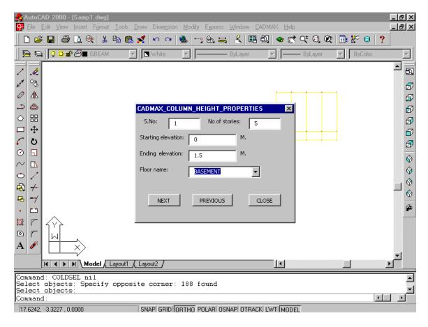
In the above dialog box, Fill the No of stories as 5 in the Textbox, and Starting elevation as 0 in the Textbox, and Ending elevation as 1.5 in the Textbox, and Floor name as "BASEMENT" from the Combo box and then press the "NEXT" button. Now you will see the same dialog box with S.No. Textbox changed automatically to 2 and remaining Textboxes such as Starting elevation, Ending elevation, Floor names are changed as follows and then "NEXT" button is pressed.
