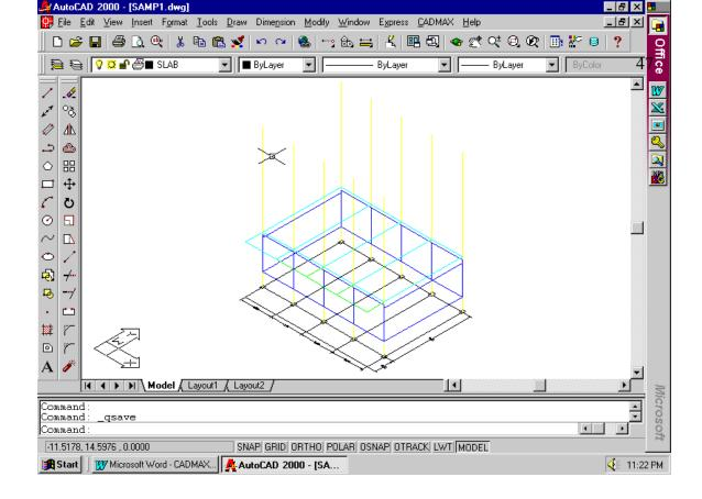
The slabs similar to the last drawn edge slab may be copied to the similar locations using array command as shown below:
