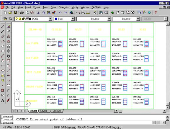
Now the detailing of columns for the structure is done. Now we can go for Detailing of beams with the following commands:
