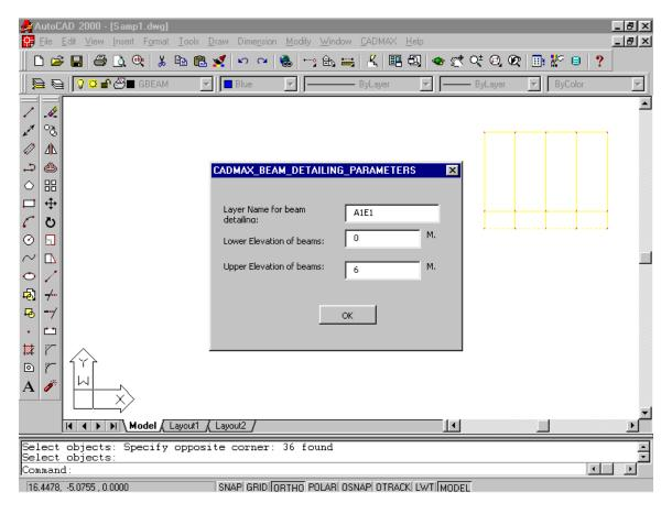
Then click OK. Now the from the selected objects only the beams within the elevation of 0 to 6m only selected for detailing and now the command prompt appears to draw the detailing of Beams selected using BEAMD command.
