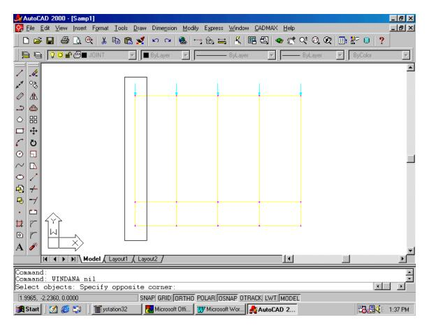
Now you will be prompted to enter Natural Ground level which is entered as 1.5m in this case and then click **OK**. Now the wind analysis for the selected frame is done. Similarly the wind analysis for the other frames are done. While designing the frame members the reversal of wind loads will be automatically considered for getting worst conditions.
