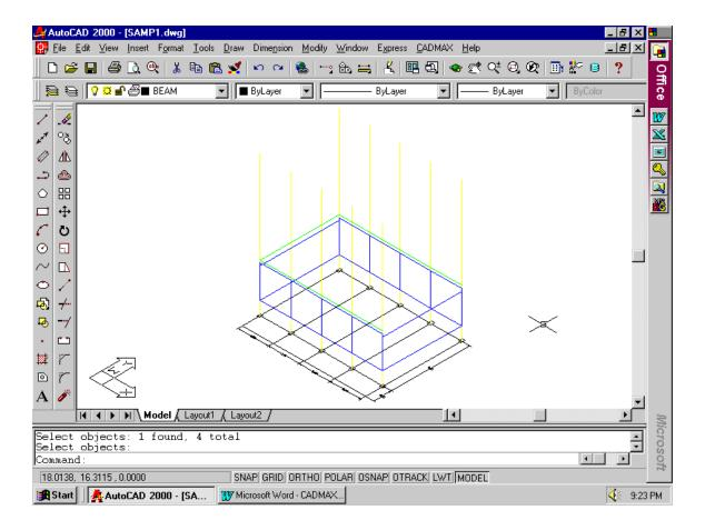
The similar beams can be copied at a distance of 3.5m c/c using array command as follows:
