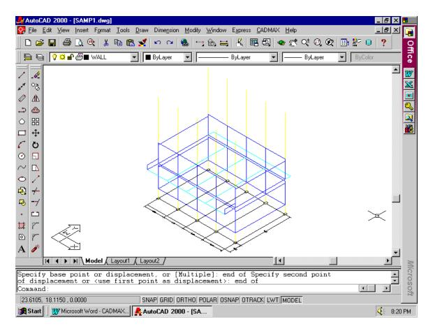
Now enter edge walls using the wall command in the same layer WALL as follows:
