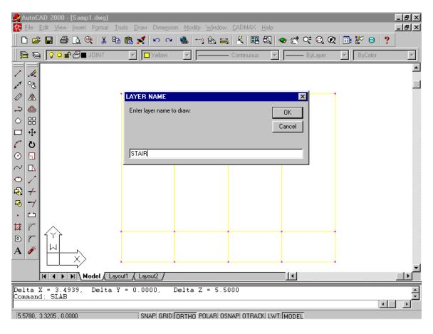
After filling the above dialog box you will be prompted for picking four corners of points and give them as previous slab commands. Then in the next dialog box select Corners at different elevations and fill them up as shown below:
