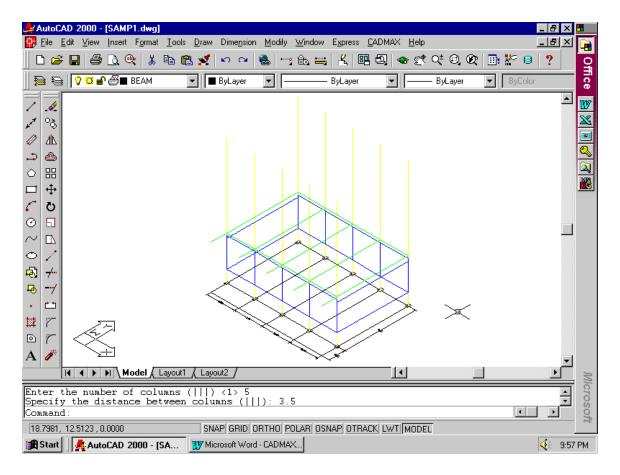
Now insert the edge beams at cantilever end points as shown below:
