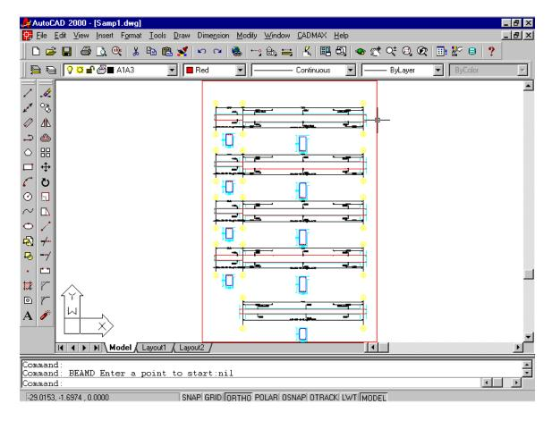
Now use Zoom All Command to go for other beam detailing and make the layer A1A3 off and set the current layer as BEAM.
