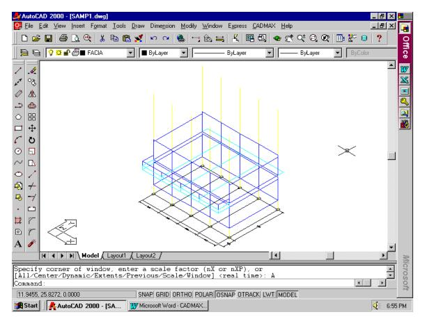
Now you can copy slabs, beams, walls, facia etc. to further floors by making off the layers "0,GBEAM,GWALL,COLUMN". The members to be copied to the other floors will be as shown below by making off the above mentioned layers.
