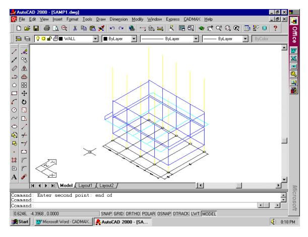
Copy the last drawn wall to the other end using copy command as done previously. Now the drawing will be seen as follows:
