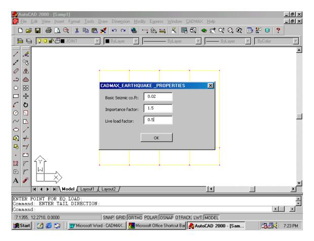
Enter the Basic seizmic co-efficient, Importance factor, and live load factor as per IS-1893 code specifications in the above dialog box and then click **OK**.
