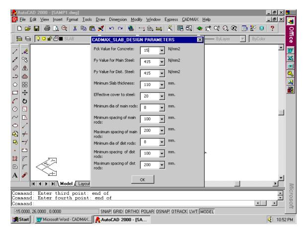
Fill in the above design parameters according to the requirements as shown above and then click **OK**.
