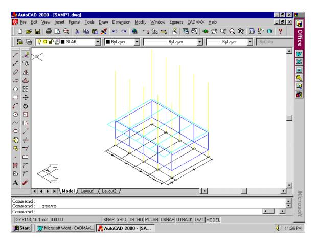
Now you can insert a cantilever slab in the rear side for a span of 1m as follows:
