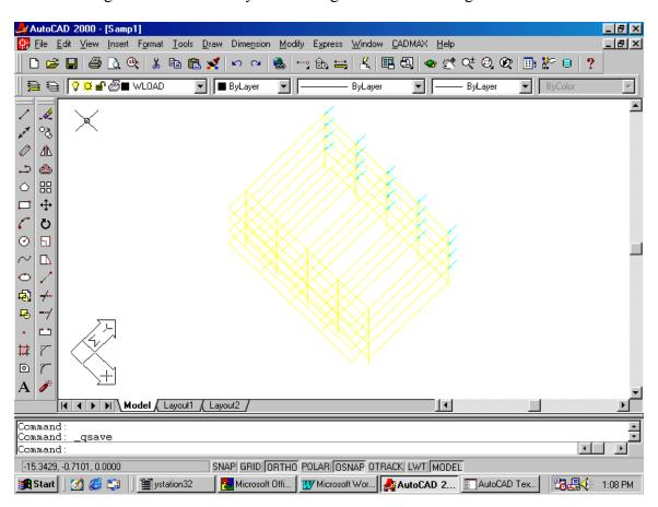
To analyse for wind load you should bring the drawing for plan view by giving vpoint as 0,0,1. Now you can do wind analysis for each frame by giving **WINDANA** command. The plan view will be as shown below:
