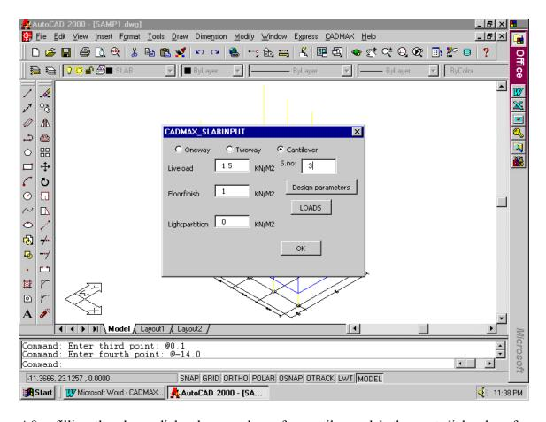
After filling the above dialog box as above for cantilever slab the next dialog box for boundary condition to select the supported edge of cantilever is displayed. In this case the first edge connecting point 1 and 2 will be the supported edge and the width of facia and height of facia and unit weight of facia are to be filled in the next dislog box as shown below:
