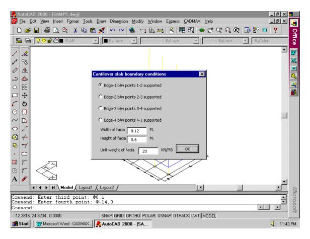
After filling in the above dialog box and then  $click\ OK$ . Now you will see the cantilever slab drawn in cyan color in the rear side of the structure.
