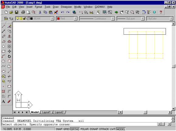
Now after selection you can use BEAMD command to detail the beams in the layer A3E3 as shown below:
