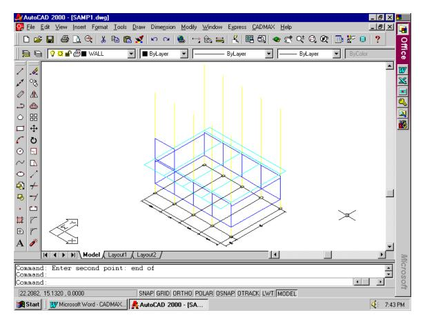
The walls similar to the last drawn can copied to the appropriate places using the array command as follows:
