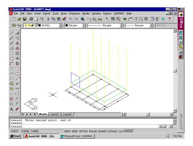
All the X-direction walls are drawn using above array command is shown below:
