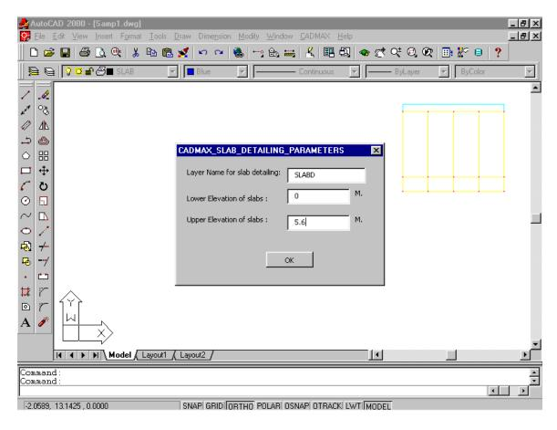
Now you asked for layer name in which the slabs are drawn using SLAB command already. In this example we have already drawn slabs in layer SLAB.
