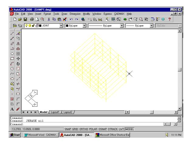
Now to analyse the structure fully use the same **ANALYSE** command. Pick the **ANALYSE** command from the **CADMAX** Popup menu Or give the **ANALYSE** command at the command prompt.
