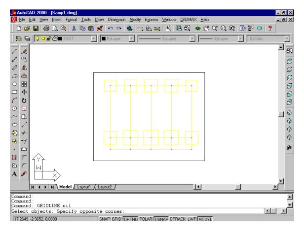
After the selection set is released, the arrangement of grid lines is finalized and saved in the drawing according to the options chosen.
