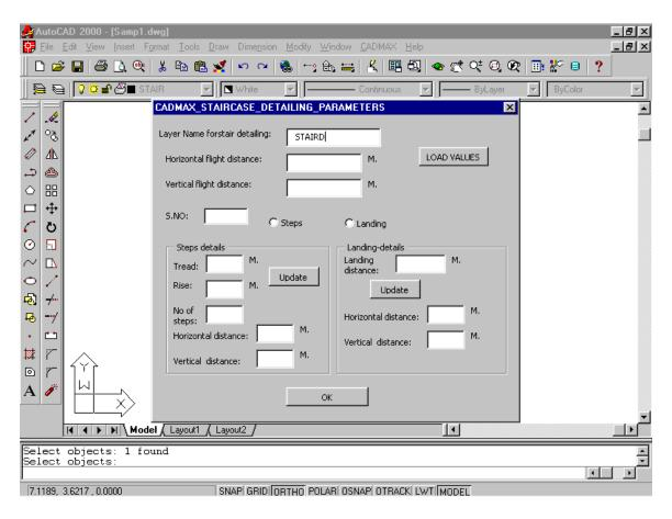
In the above dialog box you click the button LOAD VALUES and then you will see the change in dialog box with filled up values of Horizontal and Vertical distance of the flight slab is entered as shown below:
