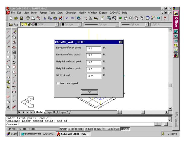
Now you will see the dialog box to fill in the wall opening details and for structural design purpose select no further openings option as follows and then click **OK**.
