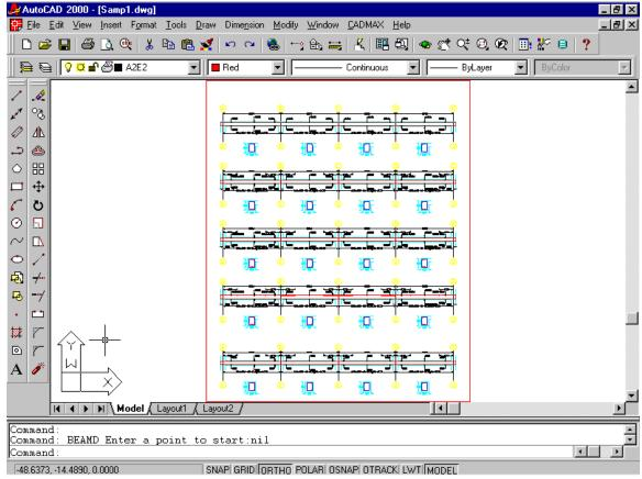
In the above drawing you are seeing the beam details of all the beams in the frame A2E2 and now use the Zoom All Command to detail further beams and make the layer A2E2 off and set the current layer as BEAM.
