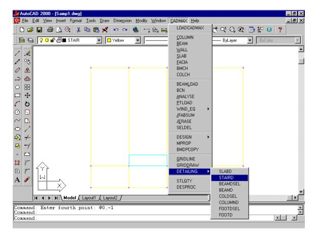
Now you will be asked to select the staircase flight slab to detail. Now select the flight slab last drawn as shown below:
