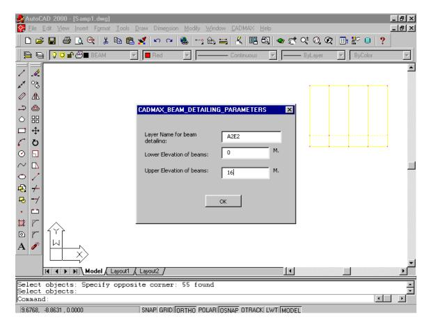
Now use the BEAMD command to draw detailing of the selected objects in layer A2E2 as shown below:
