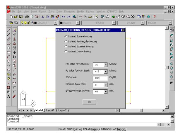
In the above Footing Design Parameters, the option box for Isolated square footings is selected and the other options will be discussed later. The Fck Value for Concrete, Fy Value for Main steel is selected from the corresponding Combo box values. The Safe Bearing Capacity of Soil is given in corresponding Text box. The Minimum dia of rods and effective cover to steel is selected from the corresponding Combo box values. Then click "**OK**" button. Now you will be prompted for Select objects.
