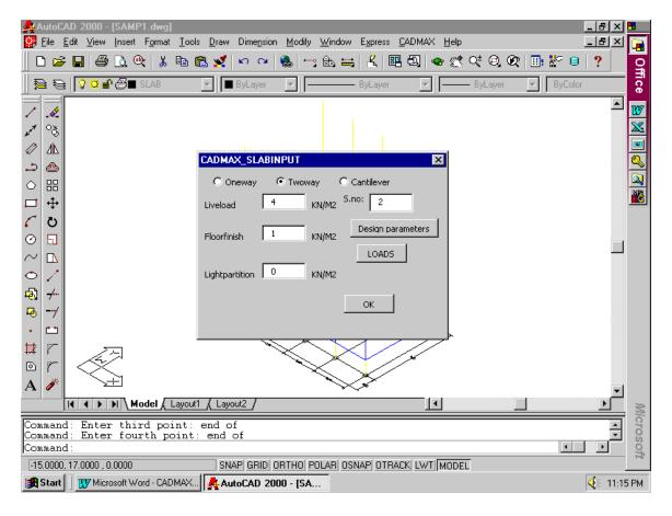
In the above dialog box fill the type of slab option as two way slab and slab no: is changed to 2 automatically and all other conditions are same and then click **OK**.
