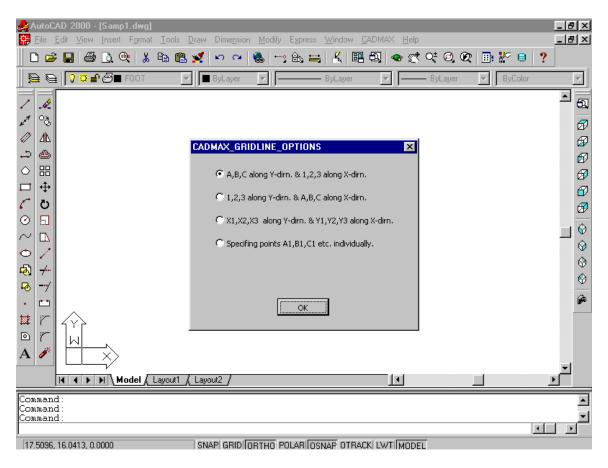
In this case the first option A,B,C numbering along X-direction and 1,2,3 numbering along Y-direction is clicked and then press "**OK**" button.
