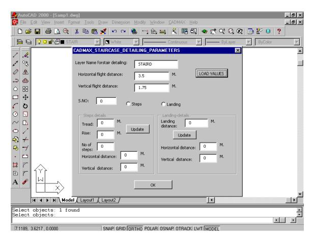
Now pick the option box Steps to draw steps first in the flight and then fill up tread and rise and No of steps as shown below:
