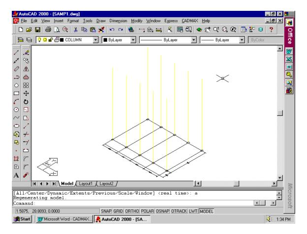
After inserting columns now you can insert grade beams at required locations.
