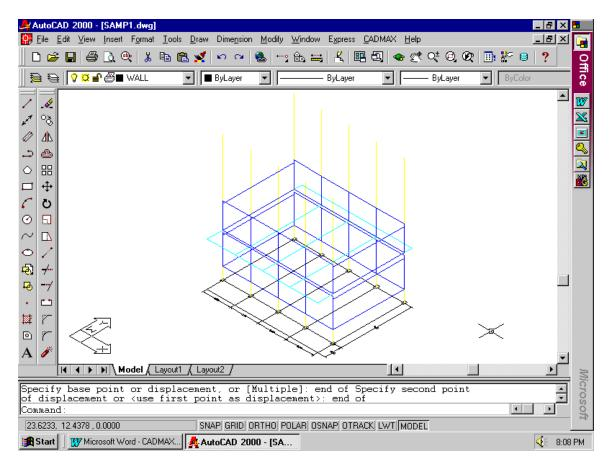
Now you can enter parapet walls in the front projections using the wall command as follows:
