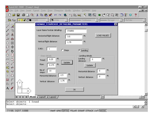
Now fill up the balance horizontal distance to be covered by landing as 1 and then click update button in landing portion as shown below:
