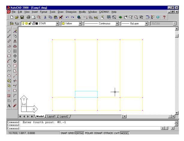
Now a Staircase flight slab is drawn as sloped slab. Now using the STAIRD command the flight slab is going to be detailed as shown below:
