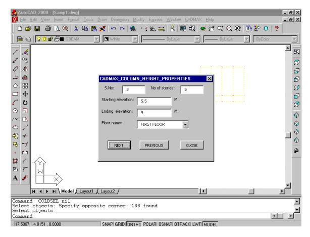
After pressing "NEXT" button, You will be prompted with the same dialog box with S.No. Textbox changed automatically to 4 and then Starting elevation, Ending elevation and Floor name are given as follows and then "NEXT" button is pressed.
