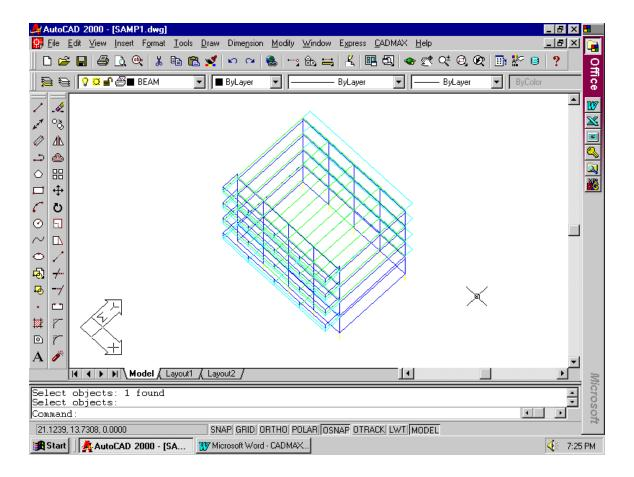
Now insert parapet walls at required places using **WALL** command from the **CADMAX** popup menu.
