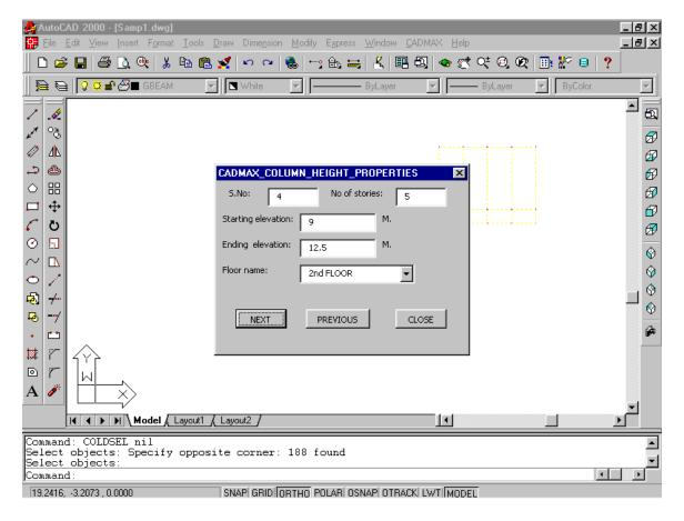
After pressing "NEXT" button, You will be prompted with the same dialog box with S.No. Textbox changed automatically to 5 and then Starting elevation, Ending elevation and Floor name are given as follows and then "NEXT" button is pressed.
