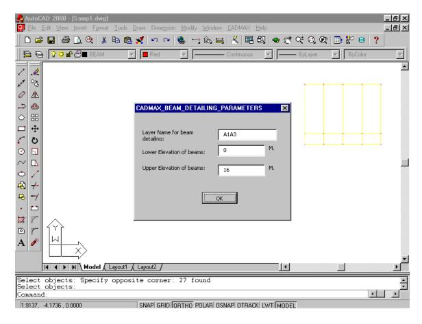
Now you can use BEAMD command to draw the beam details of selected Frame A1A3 as shown below:
