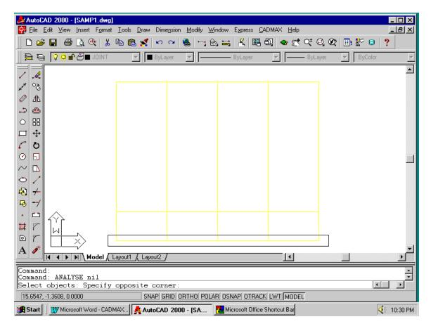
Now the edge frame is analysed within few seconds and you will see magenta color joints at the ends of beams, which shows the concentrated loads acting at the joints.
