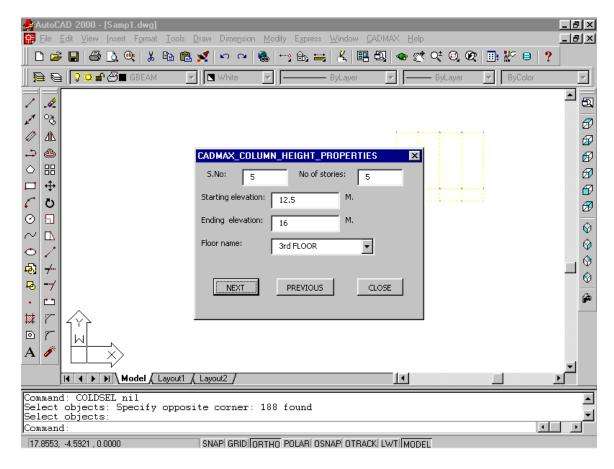
After pressing "NEXT" button you will not find change in S.No. Textbox, since the No of stories and S.No. are equal to 5. Now press "CLOSE" button. Now the dialog box will disappear. With this step the "COLDSEL" command for selection of columns for detailing is over. Now, the Column detailing is done by "COLUMND" command as follows:
