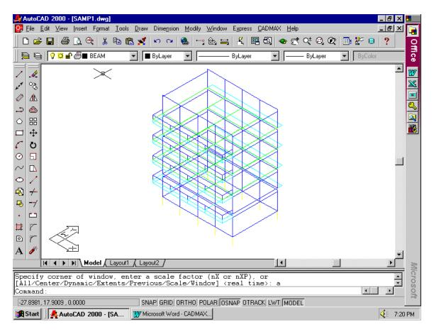
In the drawing shown now you will see high walls in the top floor instead of parapet walls. To make that changes erase high walls in the top floor and the drawing will be as shown below. To get a clear view of the structure you can give "VPOINT" command and change the vpoint as "1,-1,3" to get a following view.
