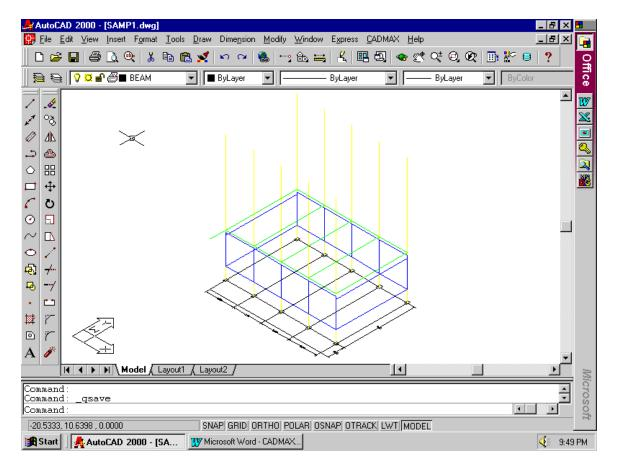
Now you can copy the last drawn cantilever beam to the appropriate locations using array command as shown below:
