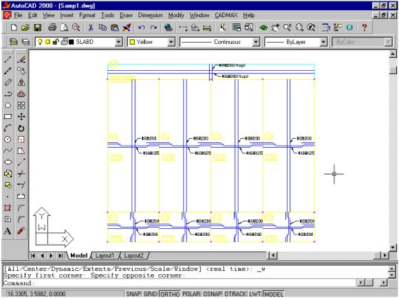
**30.STAIRD** Command: This command is used for staircase detailing.
