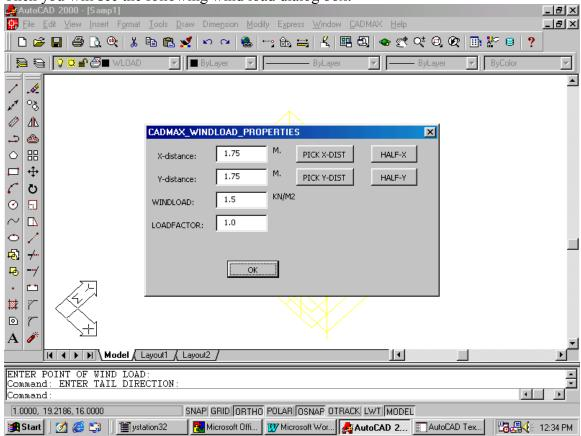
If you know the horizontal distance for wind load area you can directly fill the value in the above dialog box for X-distance as 1.75 or you can pick the button **PICK X-DIST** to specify the horizontal distance by picking the point in the drawing itself. Now you will get the following command prompt:
