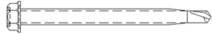
200002002 SCREW DRILL HEX HEAD M6 .3 x 1.81 x 65mm
