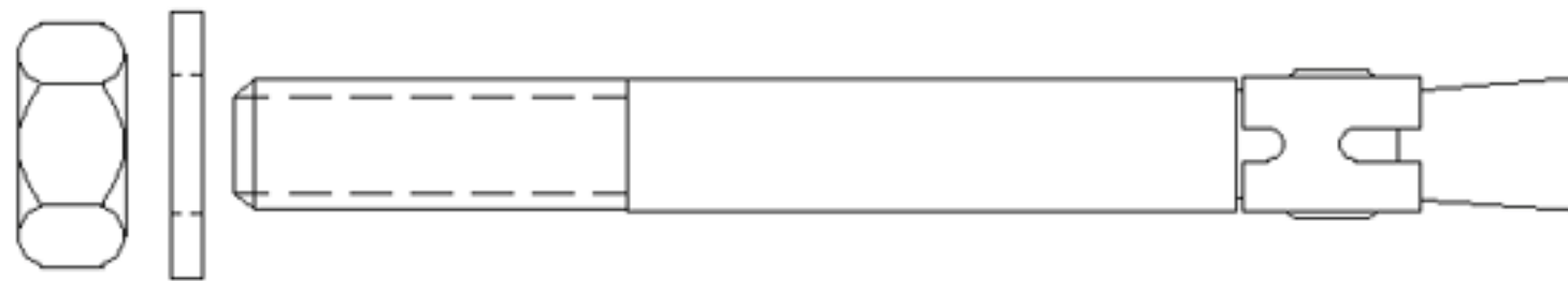
200001776 ANCHOR CONCRETE WEDGE M10 x 1.5 x 100mm
