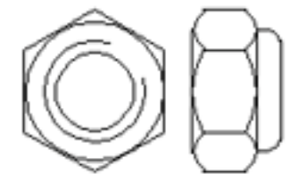
200001934 NUT LOCK HEX NYLON INSERTED M8 x 1.25
