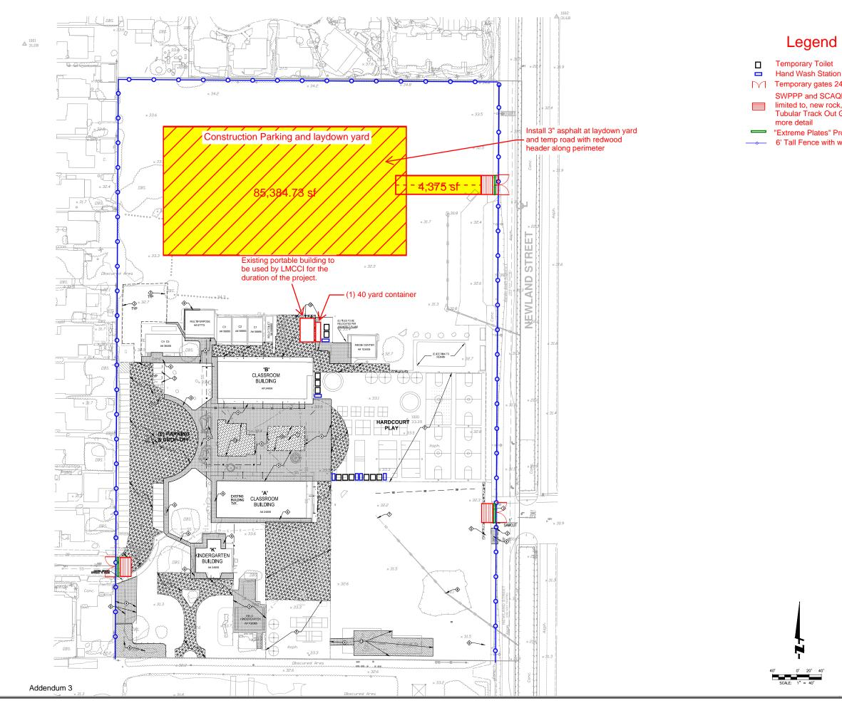
Temporary gates 24' width with hinges at each side
