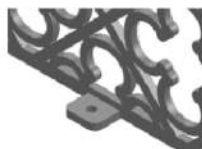
Welded on angle tabs
