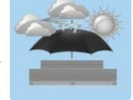
When necessary to store panels in the open, cover them completely with a white opaque polyethylene sheet or other insulating material. Cardboard cannot be exposed to moisture due to poor weathering performance and introduction of mold to the sheets and is not recomended.
