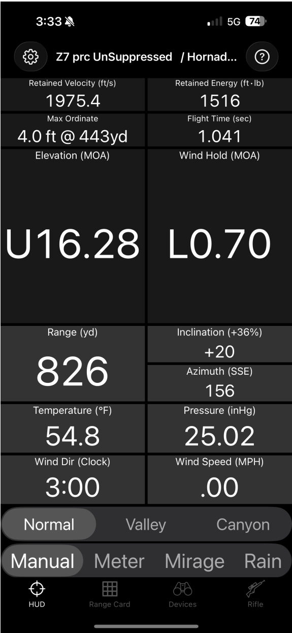
Figure 11-1. Eagle Ballistics HUD showing trajectory, target geometry, atmospheric conditions, and wind inputs.
