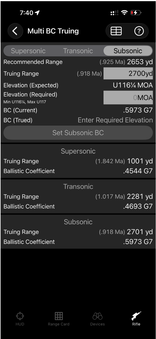
Figure 2. Multi-BC Truing screen showing the flight-region tabs, recommended range, required elevation, and stored BC values.
