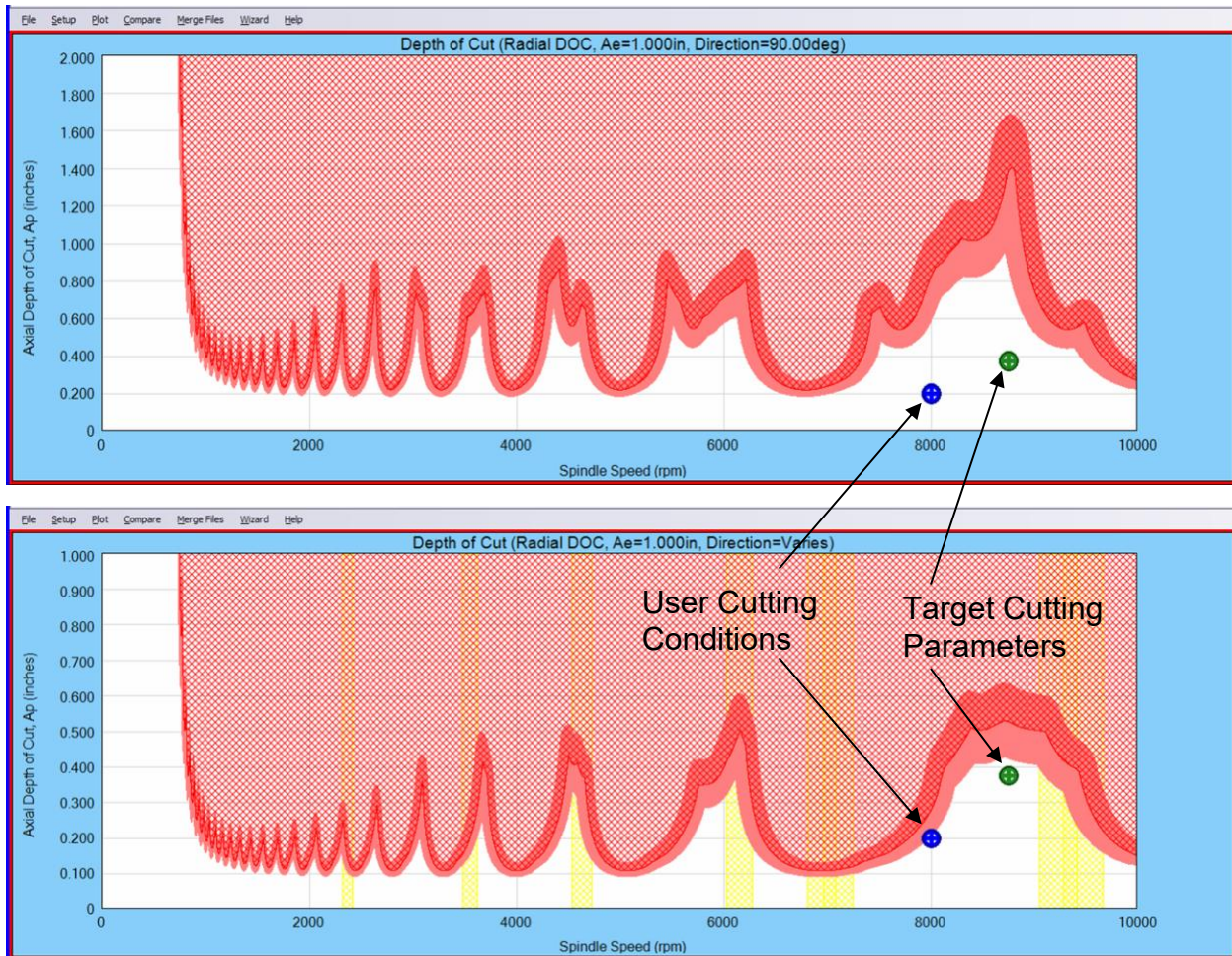
Figure 14: Stability lobe diagram for a full slot (top) for Milling Direction 90 (bottom) Sweep through milling directions using 12 steps.
