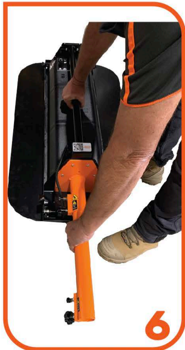
6 ATTACH TRIPOD POST TO LIGHthead
