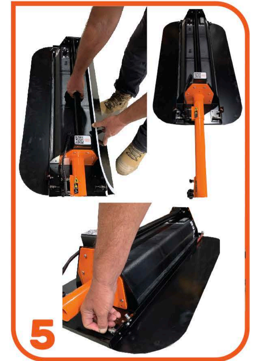
5 DETACH SIDE BOARDS FROM STOWED POSITION AND INSTALL IN OPERATIONAL POSITION FOLLOW THE COLOURS
