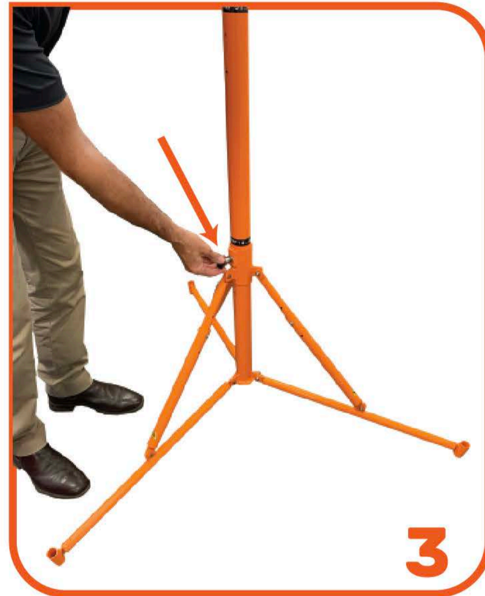
3 SLIDE TO OPEN AND LOCATE PIN ENSURE CENTER POST REMAINS OFF THE GROUND FOR STABILITY
