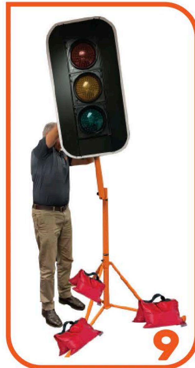
9 LIFT LIGHT HEAD INTO PLACE ON TRIPOD
