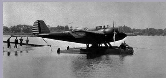
In the 1930s, Martin Aircraft put a version of their twin-engine bomber on floats. The YB-12 was a Martin B-10 with improved engines.
