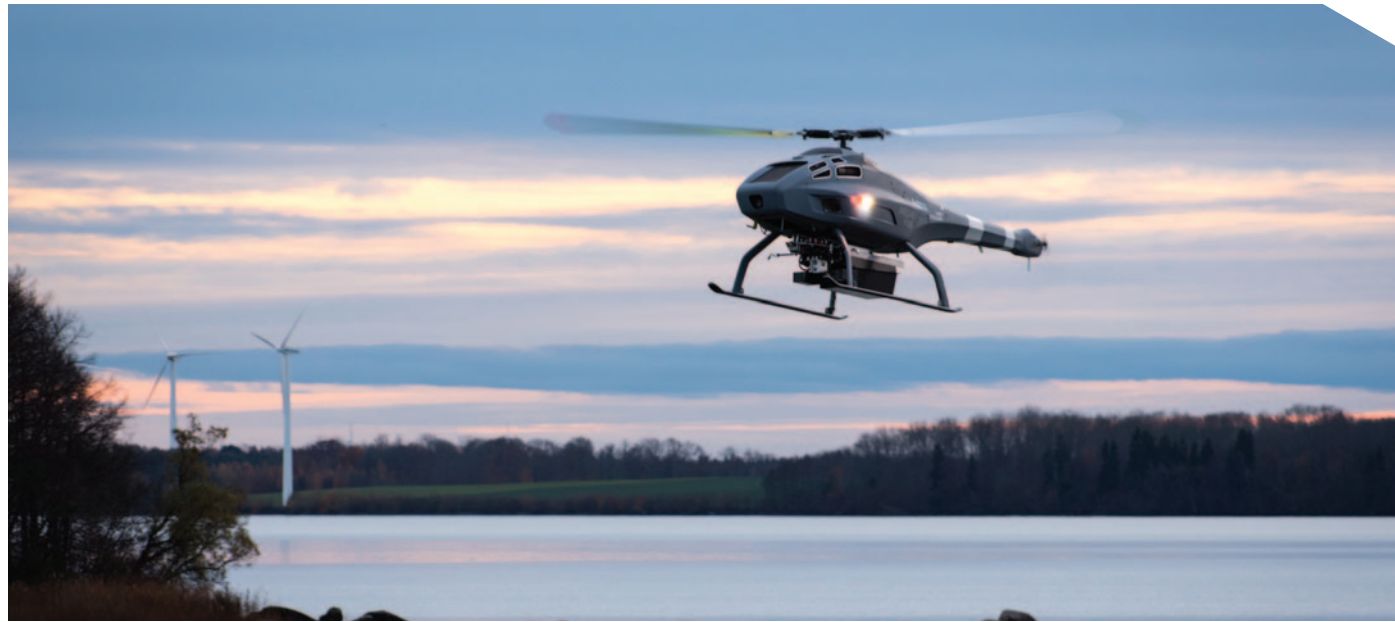
▲ A V-200 autonomous rotorcraft, equipped with a combination of sensors in a pod underneath the aircraft's body, takes off. (Photo courtesy of UMS Skeldar.)
