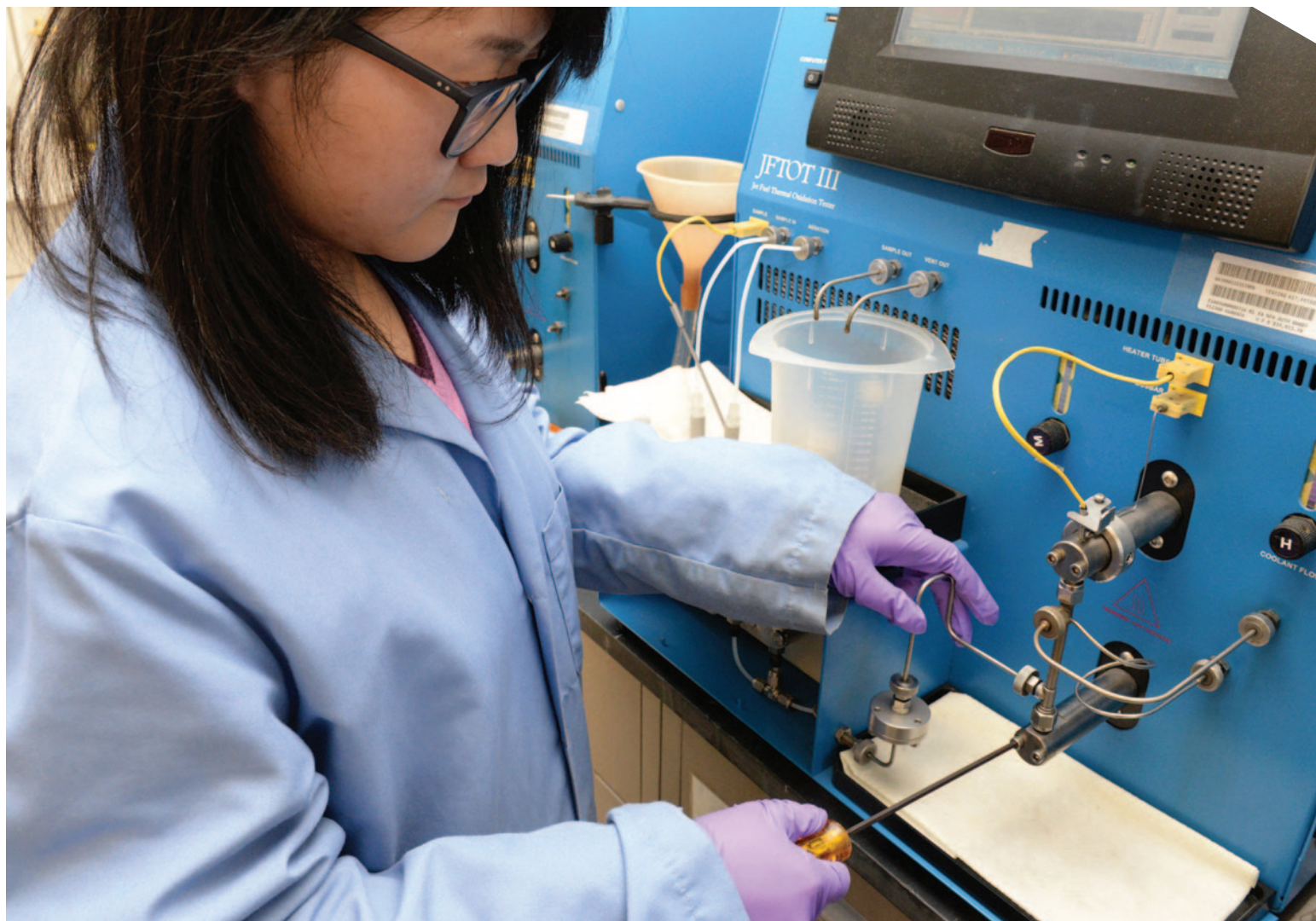
▲ Karen Kwong, U.S. Air Force Petroleum Agency chemist, prepares the Jet Fuel Thermal Oxidation Tester to run a sample in the Quality Surveillance Fuels Lab at Wright-Patterson Air Force Base, Ohio. This instrument models the conditions that fuel is exposed to inside of an aircraft during flight to determine the thermal stability of a fuel sample. Such research supports ongoing advances in reducing the carbon footprint of fleet engines. (Image courtesy of U.S. Air Force. Photo by Michelle Gigante.)
