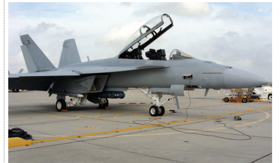
A U.S. Navy F/A-18 Super Hornet fitted with the Northrop Grumman LITENING advanced targeting pod. (Image courtesy of Northrop Grumman.)
