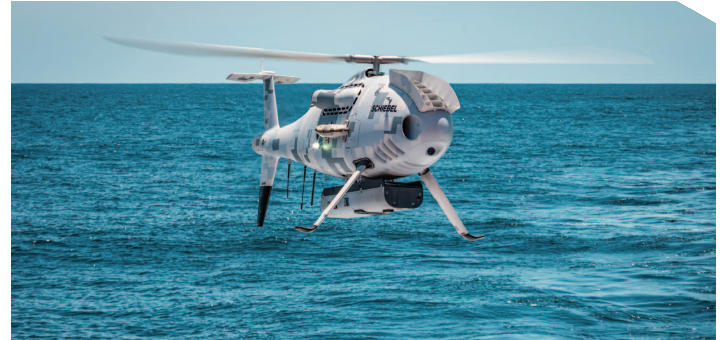
▲ The U.S. Navy held flight trials of a Camcopter, an autonomous rotorcraft, in the Gulf of Mexico. (Photo courtesy of Schiebel.)
