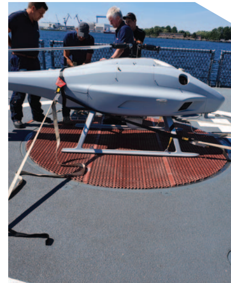
▲ Unmanned helicopters, like this V-200 undergoing a flight check, are actively being deployed on naval vessels worldwide. (Photo courtesy of UMS Skeldar.)
