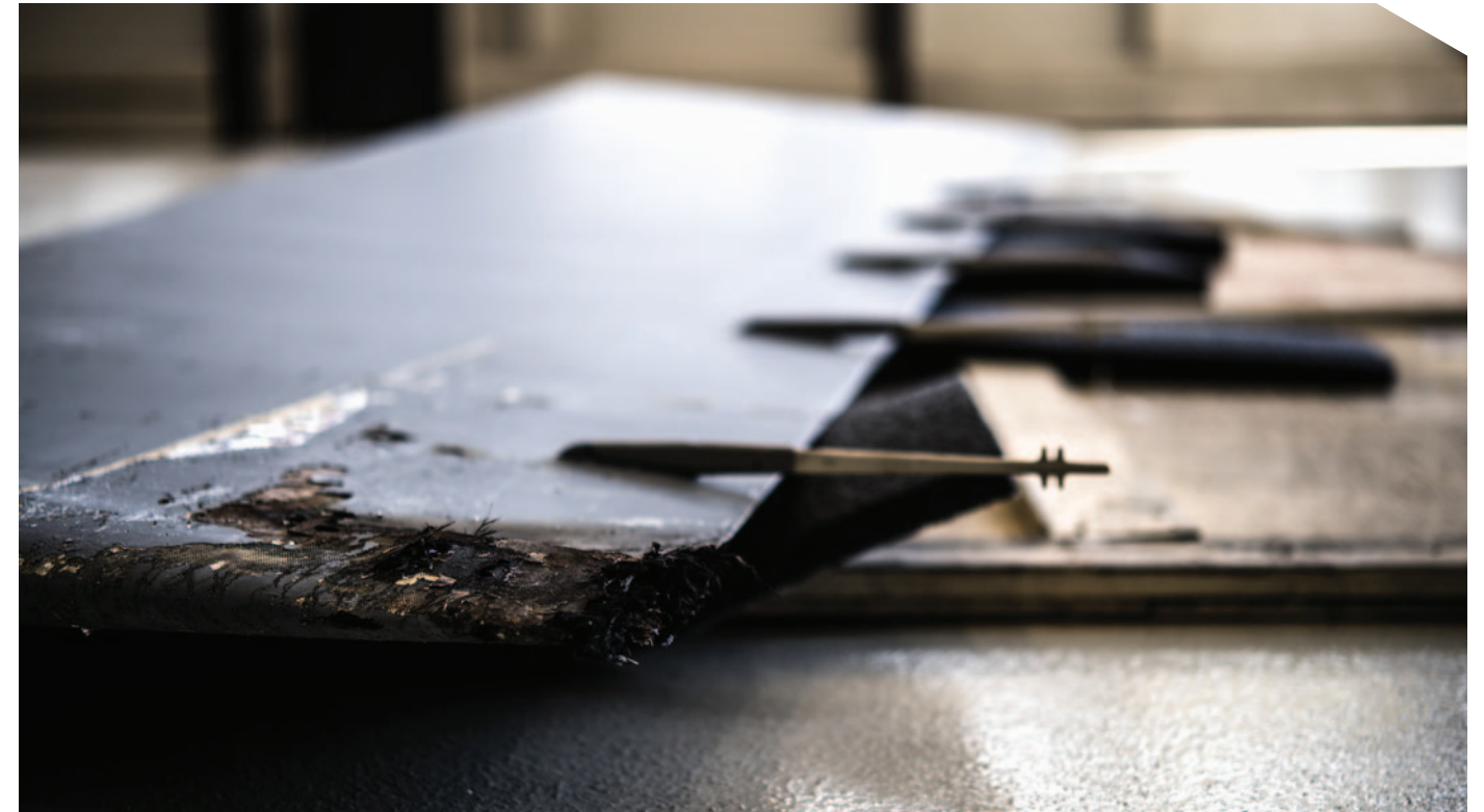
In July 2020, a bolt of lightning caused extensive structural damage to a C-17 Globemaster while flying a routine mission near Ramstein Air Base, Germany. Technicians spent 18 days repairing the aircraft to where it could be certified for a one-time flight to a structural repair facility for complete restoration. (Image courtesy of U.S. Air Force. Photo by Staff Sergeant Devin Boyer.)
