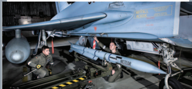
A Luftwaffe ground crew loads a Meteor BVRAAM missile aboard a Eurofighter combat aircraft. The missile is being used on Eurofighter, Gripen, and Rafale fighter aircraft and is approved for application on other advanced fighters. (Photo courtesy of MBDA Missile Systems.)
