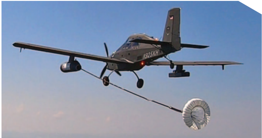
It took Northstar just eight months to develop the KC-9, a versatile refueling system for small aircraft. (Image courtesy of Northstar.)
