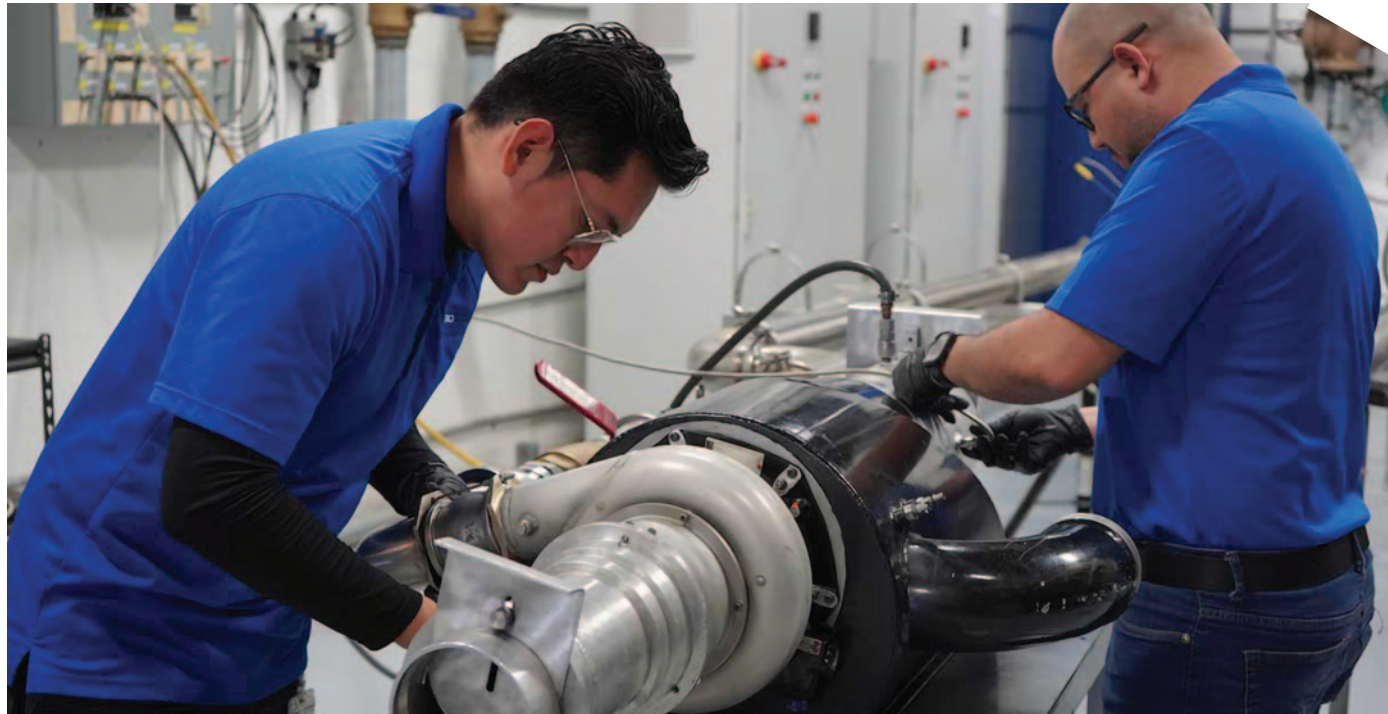
▲ This C-130J cooling turbine is being set up for a test at AeroKool. (Image courtesy of Jon Silva, AeroKool Aviation.)
