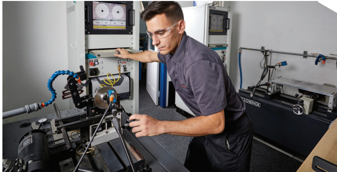
▲ An AeroKool technician balancing the shaft of an air cycle machine (ACM). (Image courtesy of Jon Silva, AeroKool Aviation.)
