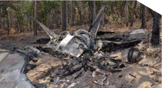
This photo shows the wreckage of an F-22 Raptor fighter jet that crashed on May 15, 2020. The cause of the crash was a small piece of tape left on the aircraft after it was washed. The tape covered a sensor, causing the aircraft to receive faulty information. This underscores the miniscule attention to detail that must go into maintaining these stealth fighters. (U.S. Air Force Times image via the Freedom of Information Act, courtesy of the U.S. Air Force.) ▼
