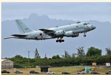
A Japan Maritime Self-Defense Force P-1 patrol aircraft takes off from U.S. Marine Corps Air Station Kaneohe Bay, Hawaii, during Exercise Rim of the Pacific (RIMPAC) 2024. The Kawasaki P-1 is the currently the only production military aircraft that uses a fiber optic “fly-by-light” flight control system. (Japan Maritime Self-Defense Force photo by Petty Officer 2nd Class Atsushi Mashima.)
