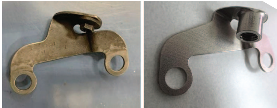
▲ Pratt & Whitney produced a loop bracket for the TF33 engine conventionally (at left) and used additive manufacturing (at right) to redesign and produce it for installation on a U.S. Air Force B-52H Stratofortress. (Photo courtesy of Pratt & Whitney.)
