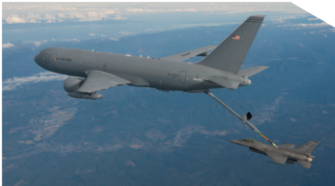
A Boeing KC-46 Pegasus uses a boom to refuel a U.S. Air Force F-16 built by Lockheed Martin. (Image courtesy of Boeing.)
