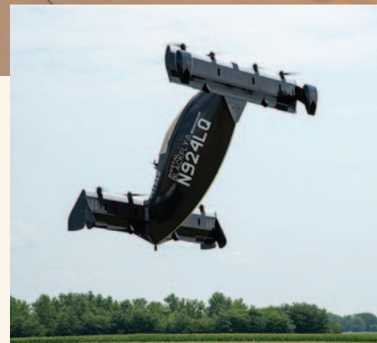
Pivotal's BlackFly electric vertical take-off and landing, or eVTOL, aircraft, along with other electric aircraft, is shown being evaluated during Exercise AGILE FLAG 24-3, held in California in August. Tests were conducted in an unmanned configuration to better assess aircraft potential capabilities, including complex remote and autonomous systems controls. (Image courtesy of the U.S. Department of Defense.)
