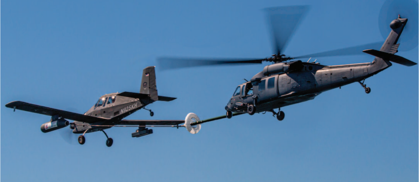
A small airplane equipped with Northstar's aerial refueling system has the ability to match airspeed with other small planes, various UAVs, and helicopters. (Image courtesy of Northstar.)
