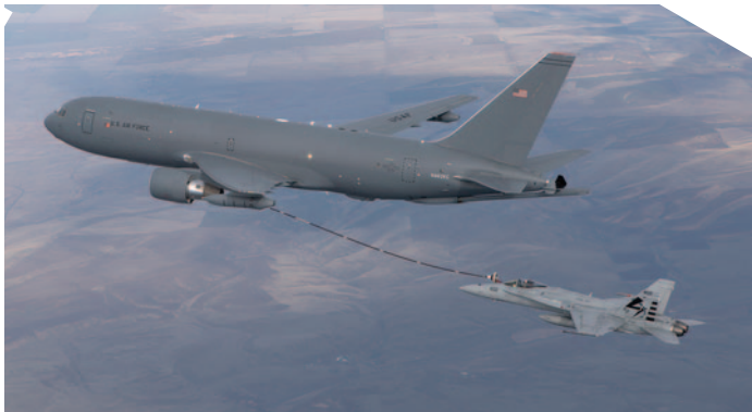
U.S. Navy fighters such as the F-18 are designed to receive fuel through a probe-and-drogue system. (Image courtesy of Boeing.)
