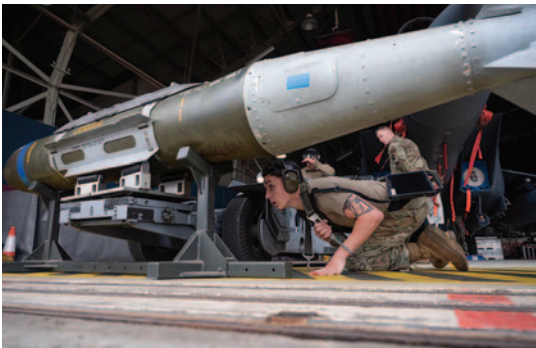
A Joint Direct Attack Munition GBU-31 is shown during an exercise. Bolt-on attachments, which convert a gravity bomb into a precision-targeted one, are visible. (U.S. Air Force photo by Senior Airman Koby I. Saunders.)
