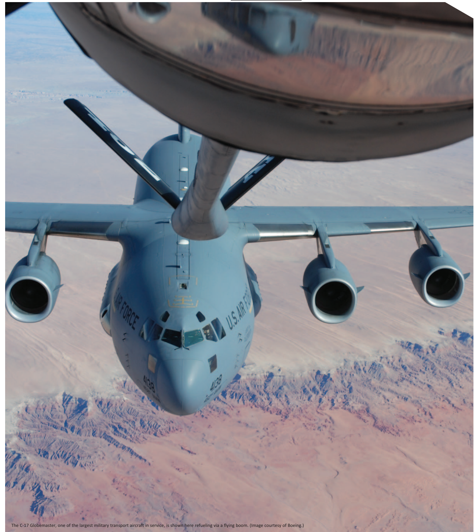
The C-17 Globemaster, one of the largest military transport aircraft in service, is shown here refueling via a flying boom. (Image courtesy of Boeing.)
