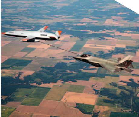
▲ The Boeing MQ-25 Stingray aerial refueling drone is designed to operate from U.S. Navy aircraft carriers. Here, it is shown refueling an F-35C. (Image courtesy of Boeing.)
