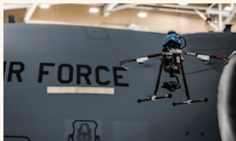
The 911th Maintenance Squadron at the Pittsburgh International Airport Air Reserve Station, Pennsylvania, uses a small drone to conduct inspections of hard-to-reach parts of a Globemaster. (U.S. Air Force photo by Joshua J. Seybert.)
