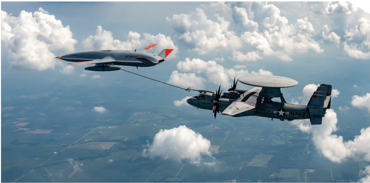
▲ An MQ-25 Stingray refuels an E-2D Advanced Hawkeye over MidAmerica Airport, Mascoutah, Illinois, in August 2021. The second successful refueling by an unmanned MQ-25, this test flight evaluated fuel transfer, formation flying, wake turbulence, drogue tracking, and in-flight connections. (U.S. Navy photo courtesy of Boeing.)
