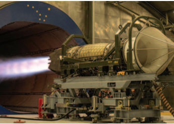
A Pratt & Whitney F119-PW-100 turbofan engine run is conducted at Joint Base Elmendorf-Richardson, Alaska. (U.S. Air Force photo by Airman First Class Andrew Britten.)
