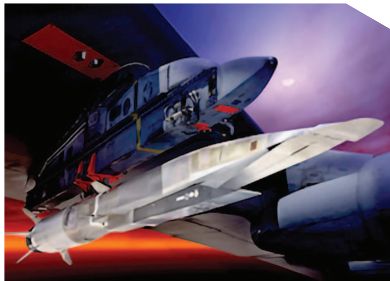
▲ The X-51A Waverider, shown here under the wing of a B-52 Stratofortress, is set to demonstrate hypersonic flight. Powered by a Pratt & Whitney Rocketdyne SJX61 scramjet engine, the missile is designed to ride on its own shockwave and accelerate to about Mach 6. (Image courtesy of the U.S. Air Force.)
