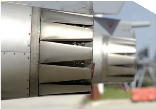
Two EJ200 engines, each providing 20,000 pounds of thrust, give the Typhoon a top speed of more than Mach 2. (Image courtesy of Geoffrey Lee/Eurofighter.)
