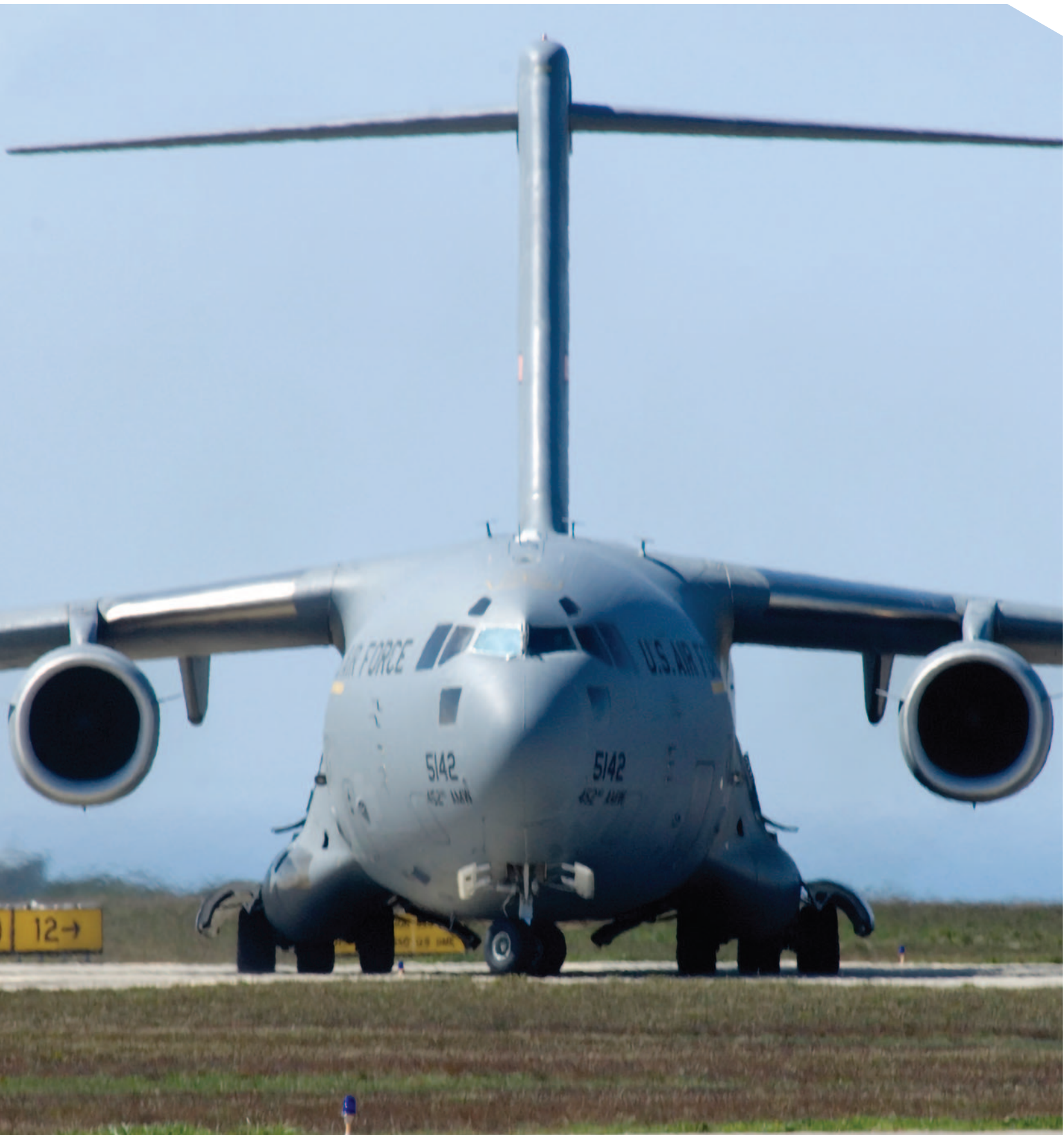
A C-17 Globemaster III, stationed at March Air Reserve Base, Calif., performs a reverse thrust maneuver for training at Vandenberg Air Force Base, CA. A thin water vapor vortex appears on the far left engine. (U.S. Air Force photo/Staff Sgt. Levi Riendeau)
