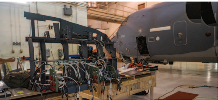
A combat systems officer station shell sits on a table at Moody Air Force Base, Georgia. The station and software upgrades will support Link 16, a tactical data network system that can establish communication between aircraft for a full picture of a battlespace. (U.S. Air Force photo by Senior Airman Deanna Muir.)
