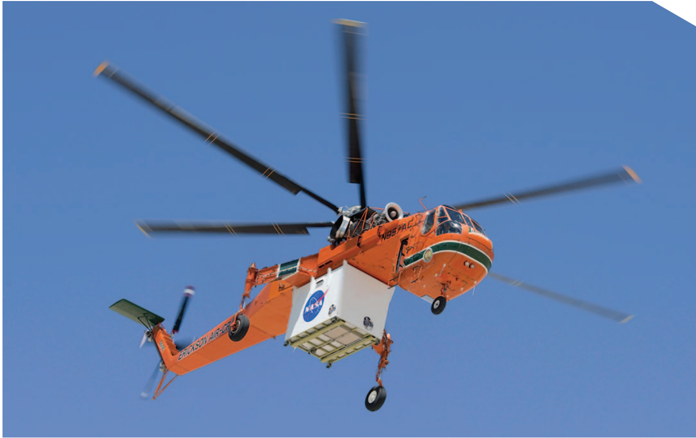
▲ An Erickson Air-Crane helicopter departs on an Autonomous Landing and Hazard Avoidance Technology (ALHAT) LiDAR test flight from NASA's Dryden Flight Research Center in July 2010. The flight-tested terrain recognition and LiDAR systems were developed by NASA Langley and Jet Propulsion Laboratory to enable safe landings. (NASA photo by Tony Landis.)
