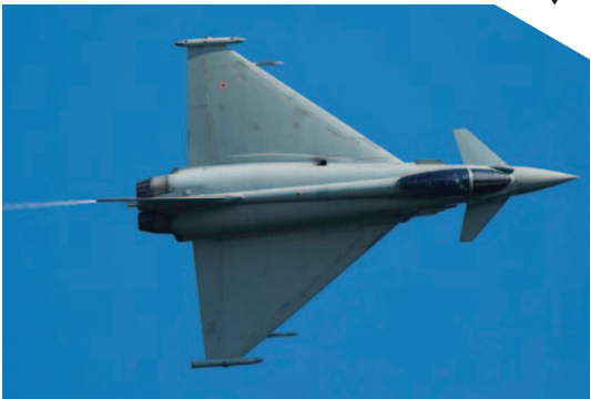
The Typhoon is instantly recognizable in the sky, due to its delta wing design and distinctive canards. (Image courtesy of Geoffrey Lee/Eurofighter.)
